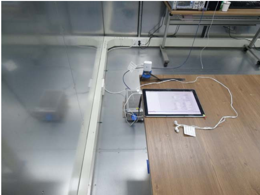
LINE CONDUCTED BACK PHOTO
