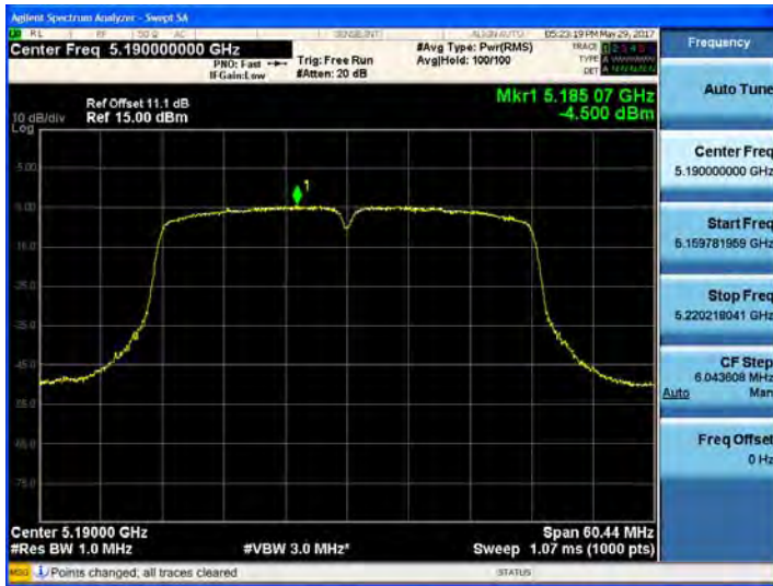
802.11n_HT40 UNII 2C BAND PSD CH 134
