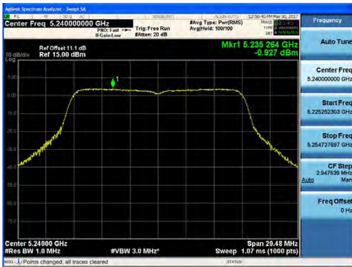
802.11n_HT20 UNII 2C BAND PSD CH 140
