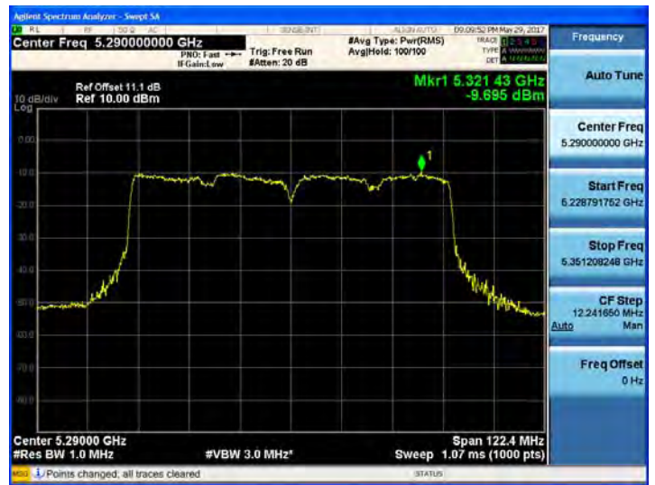
802.11ac_VHT80 UNII 3 BAND PSD CH 155
