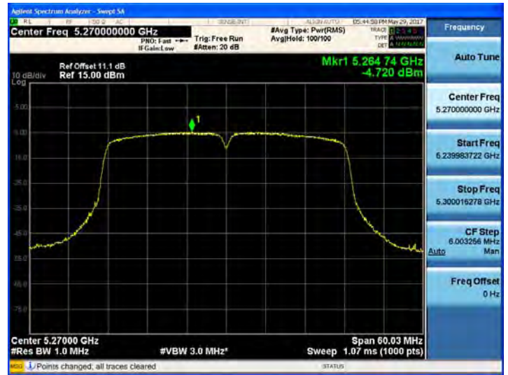
802.11n_HT40 UNII 3 BAND PSD CH 151
