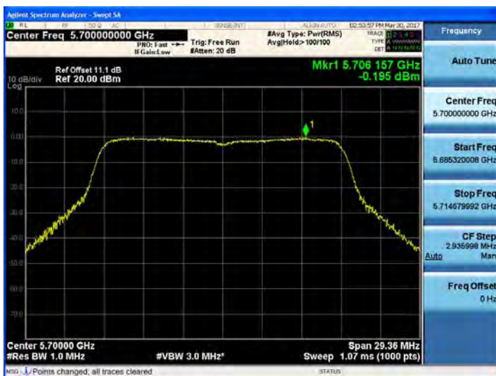
802.11n_HT20 UNII 2C BAND PSD CH 140
