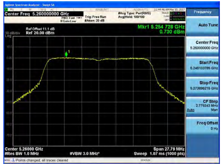
802.11a UNII 3 BAND PSD CH 165
