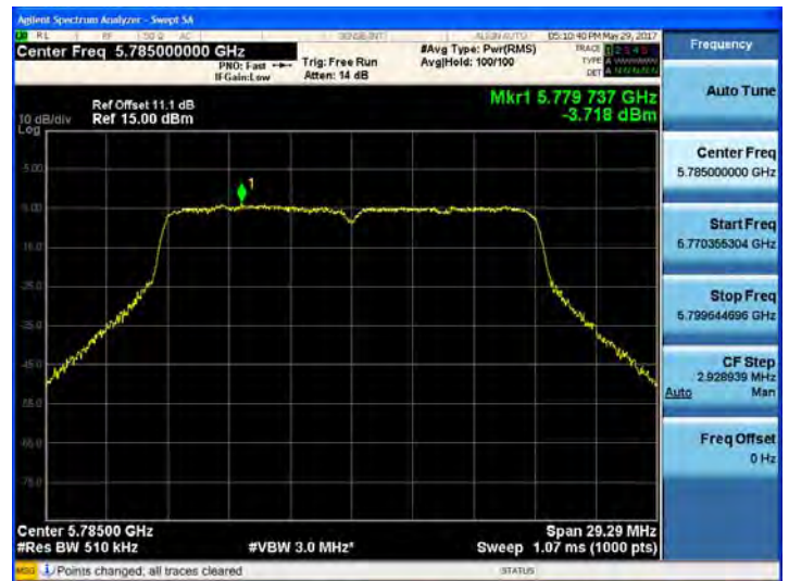
802.11ac_VHT20 UNII 3 BAND PSD CH 157
