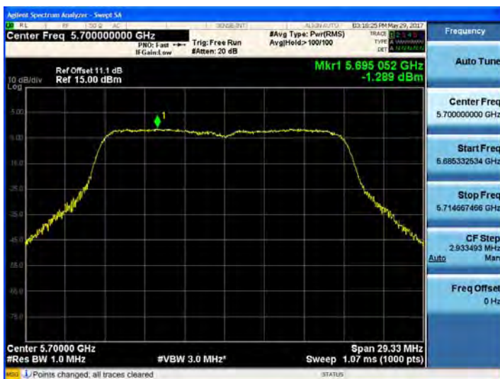
802.11n_HT20 UNII 2C BAND PSD CH 140
