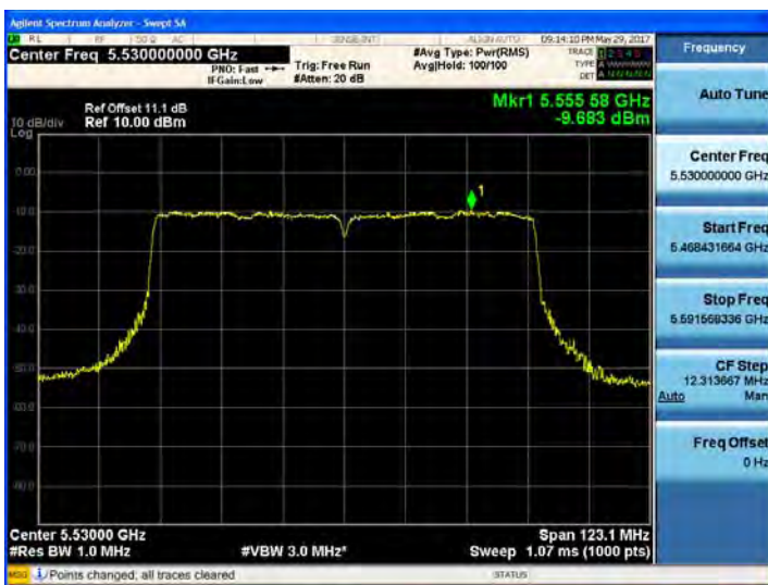
802.11ac_VHT80 UNII 2C BAND PSD CH 106
