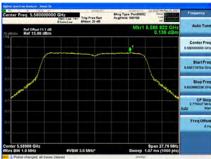
802.11a UNII 2C BAND PSD CH 116
