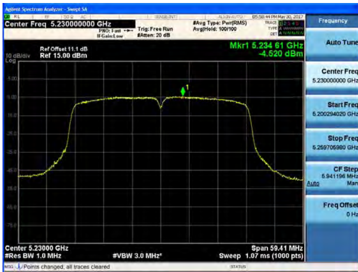
802.11ac_VHT40 UNII 2C BAND PSD CH 134
