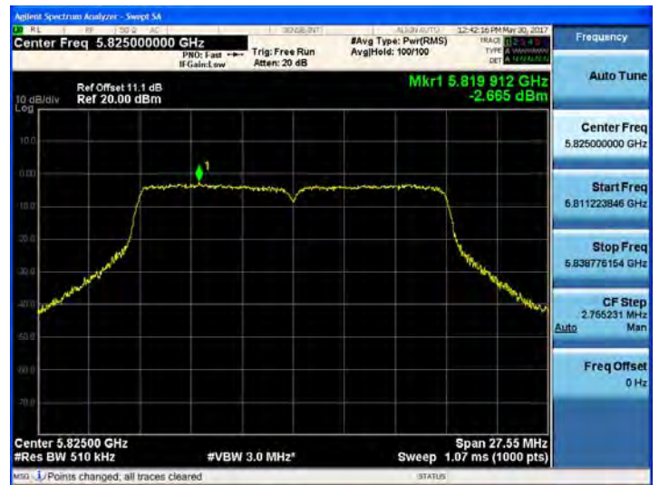
802.11a UNII 3 BAND PSD CH 165
