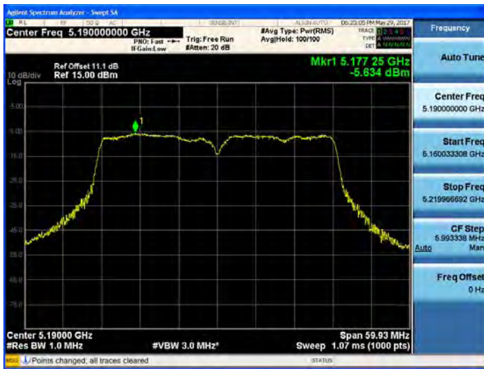
802.11ac_VHT40 UNII 2C BAND PSD CH 134
