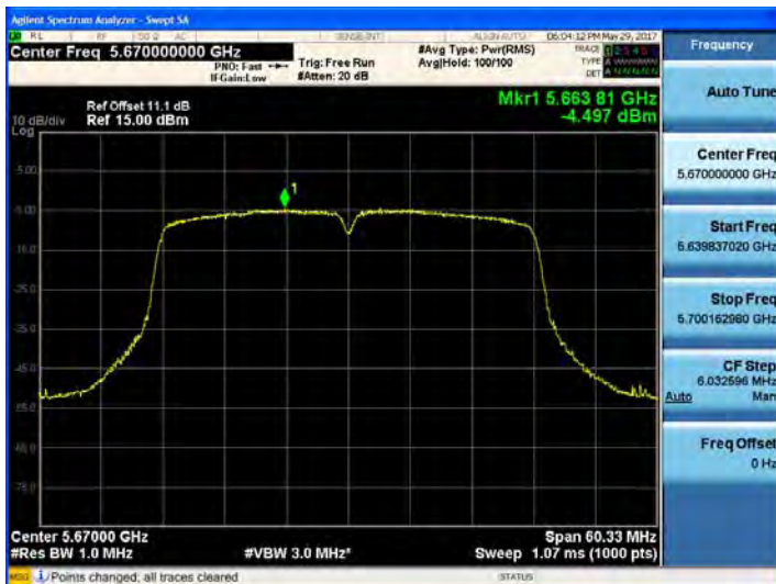
802.11n_HT40 UNII 2C BAND PSD CH 134
