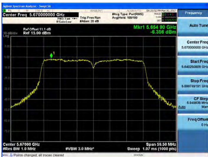
802.11ac_VHT40 UNII 2C BAND PSD CH 134
