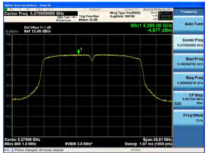
802.11ac_VHT40 UNII 3 BAND PSD CH 159
