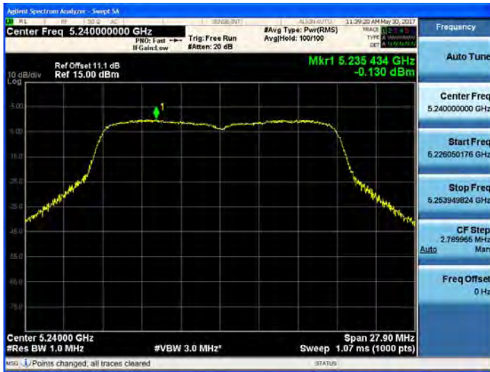
802.11a UNII 2C BAND PSD CH 140
