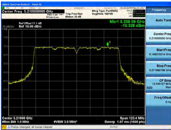
802.11ac_VHT80 UNII 2C BAND PSD CH 106
