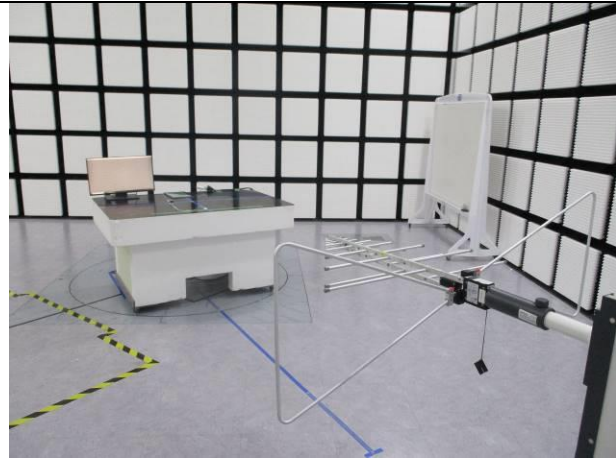
RADIATED FRONT PHOTO (BELOW 1 GHz)
