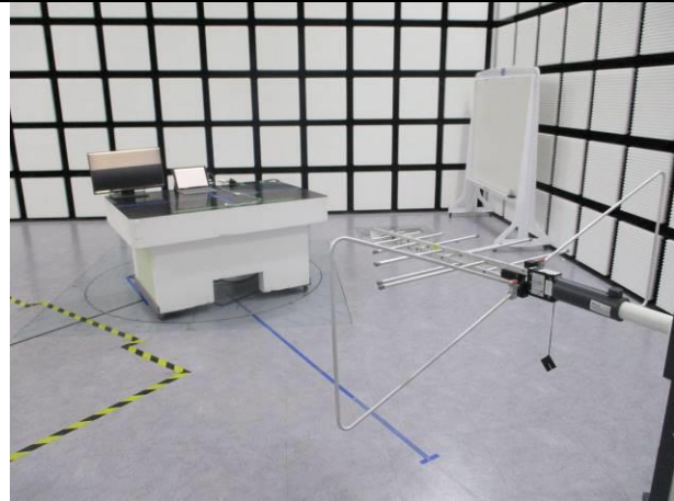
RADIATED FRONT PHOTO (BELOW 1 GHz)
