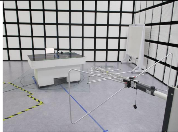
RADIATED FRONT PHOTO (BELOW 1 GHz)
