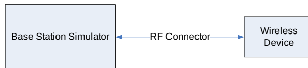
Figure 10-2 Power Measurement Setup
