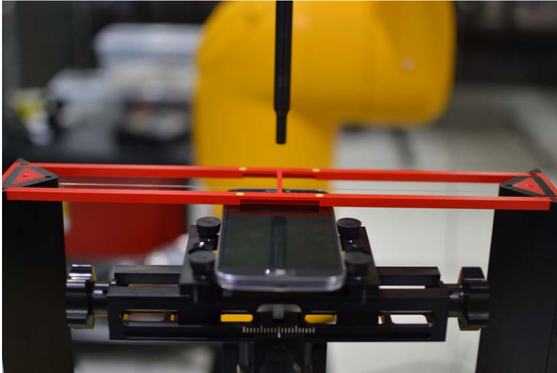
Figure 18-1 Ear Reference Point HAC Phantom Alignment
