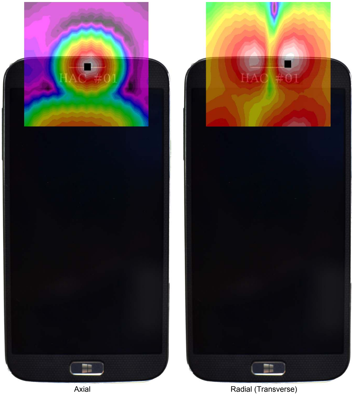
Figure 13-3 T-Coil Scan Overlay Magnetic Field Distributions
