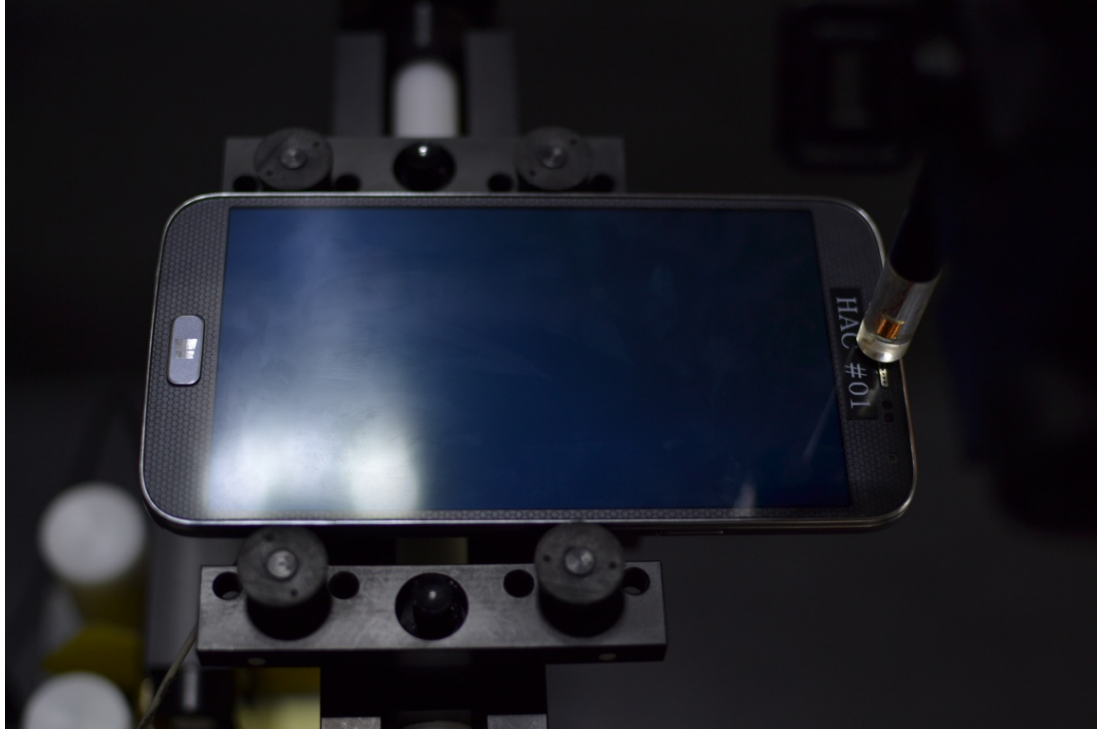
Figure 13-1 Test Setup for Wireless Device
