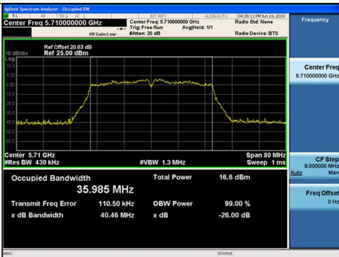
802.11ac_VHT40 UNII 2C BAND 26dB Bandwidth(CH 142)
