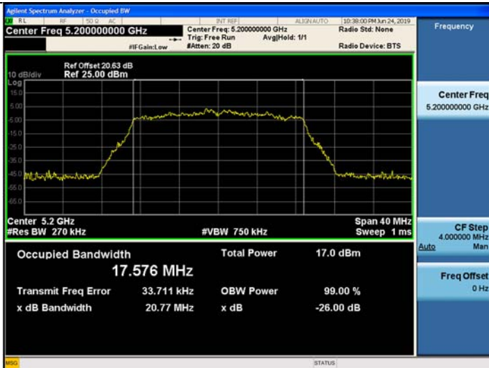
802.11ac_VHT20 UNII 2C BAND 26dB Bandwidth(CH 100)
