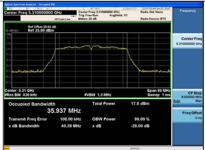
802.11n_HT40 UNII 3 BAND 26dB Bandwidth (CH 151)
