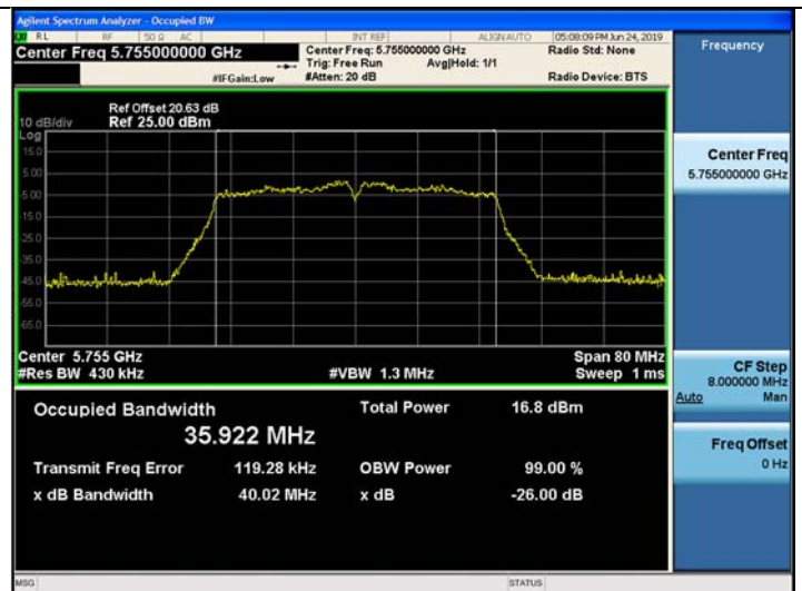
802.11ac_VHT40 UNII 3 BAND 26dB Bandwidth (CH 151)
