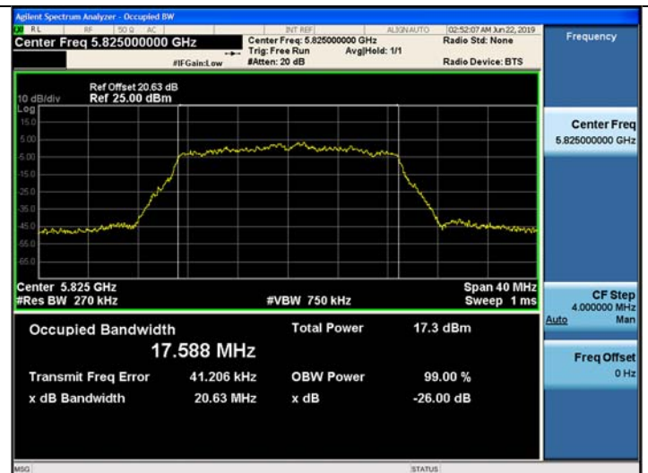
802.11ac_VHT20 UNII 3 BAND 26dB Bandwidth(CH 165)
