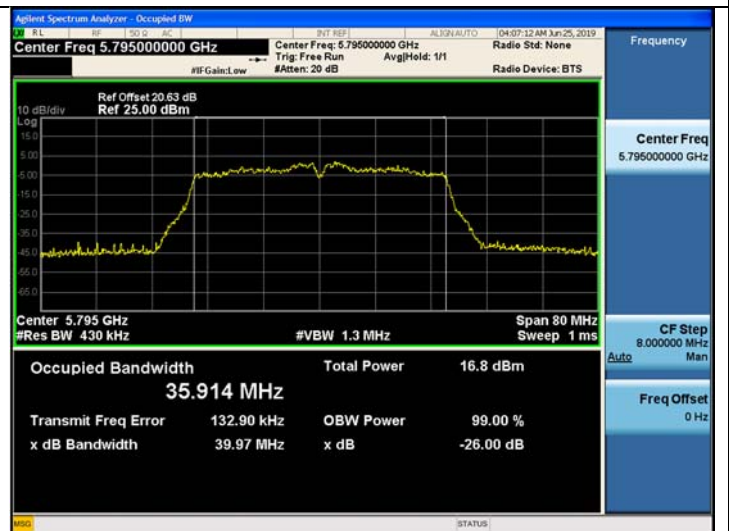
802.11ac_VHT40 UNII 3 BAND 26dB Bandwidth (CH 159)
