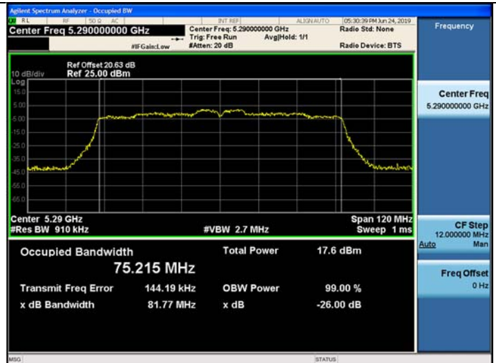
802.11ac_VHT80 UNII 3 BAND 26dB Bandwidth (CH 155)
