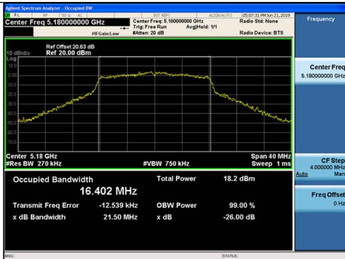
802.11a UNII 2C BAND 26dB Bandwidth (CH120)
