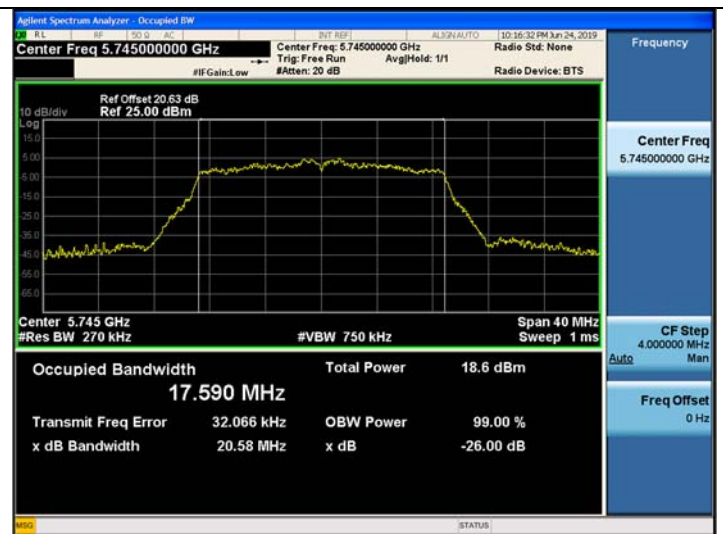
802.11n_HT20 UNII 3 BAND 26dB Bandwidth(CH 149)
