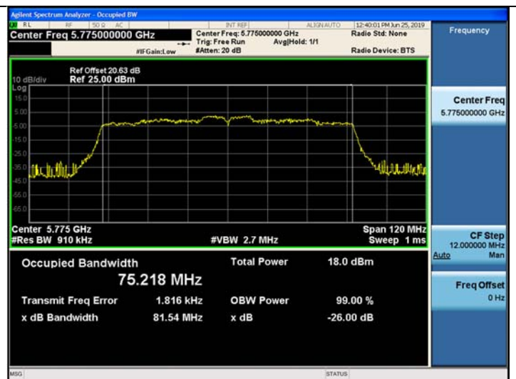
802.11ac_VHT80 UNII 3 BAND 26dB Bandwidth (CH 155)
