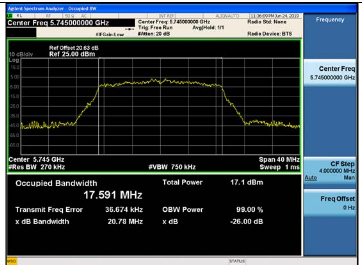
802.11ac_VHT20 UNII 3 BAND 26dB Bandwidth(CH 149)
