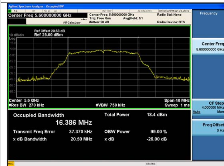
802.11a UNII 2C BAND 26dB Bandwidth (CH120)
