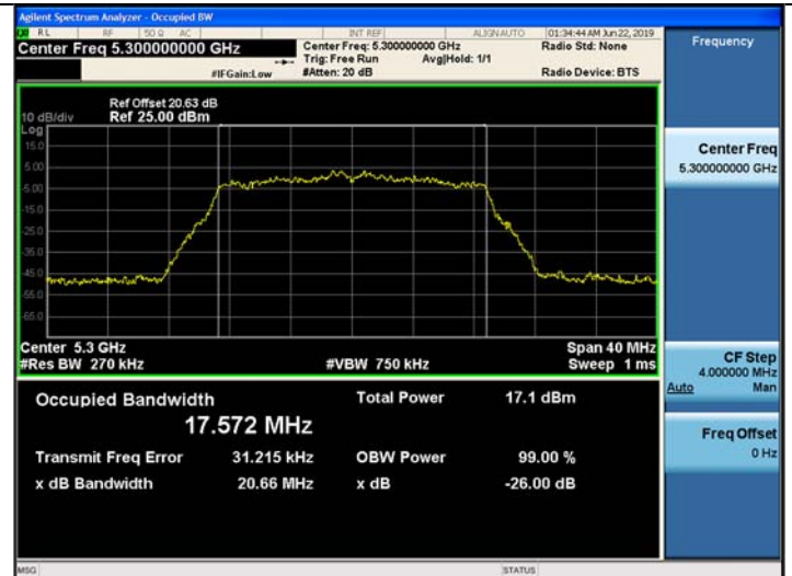
802.11ac_VHT20 UNII 3 BAND 26dB Bandwidth(CH 165)
