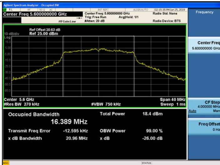
802.11a UNII 2C BAND 26dB Bandwidth (CH120)
