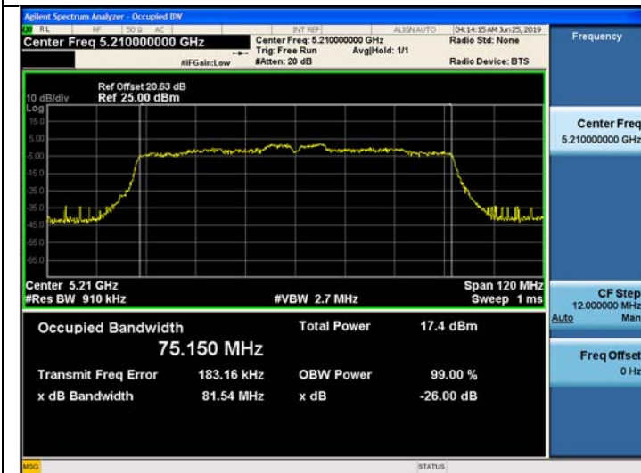
802.11ac_VHT80 UNII 2C BAND 26dB Bandwidth(CH 106)
