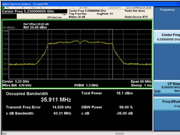
802.11n_HT40 UNII 2C BAND 26dB Bandwidth(CH 142)
