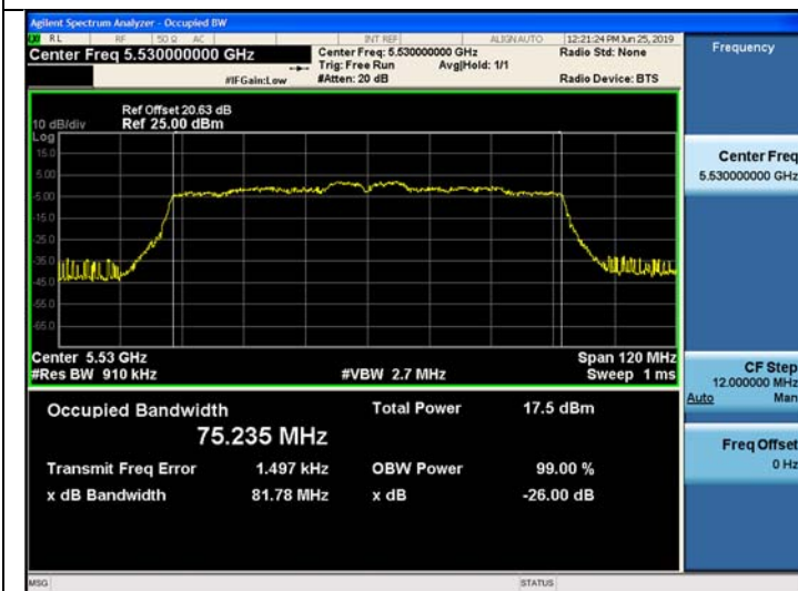
802.11ac_VHT80 UNII 2C BAND 26dB Bandwidth(CH 106)
