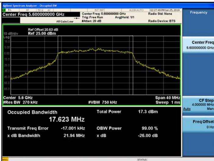
802.11ac_VHT20 UNII 2C BAND 26dB Bandwidth(CH 120)
