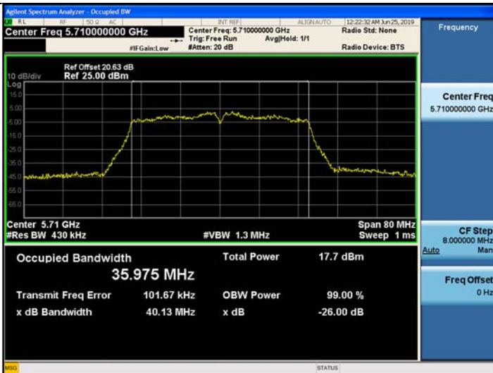
802.11n_HT40 UNII 2C BAND 26dB Bandwidth(CH 142)
