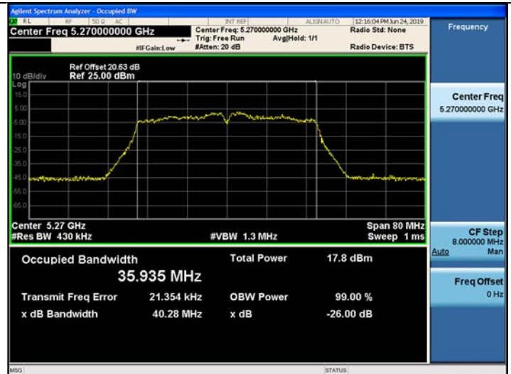
802.11n_HT40 UNII 3 BAND 26dB Bandwidth (CH 159)
