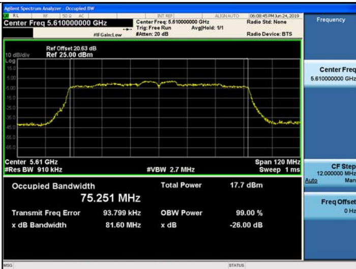
802.11ac_VHT80 UNII 2C BAND 26dB Bandwidth(CH 122)
