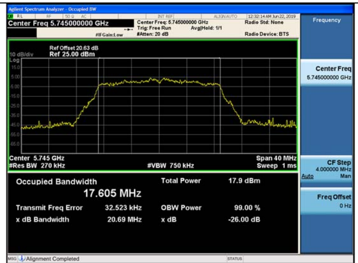
802.11n_HT20 UNII 3 BAND 26dB Bandwidth(CH 149)
