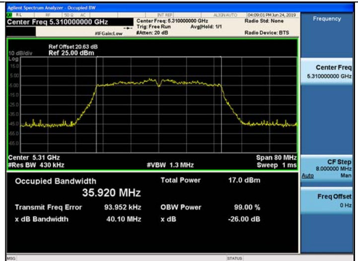
802.11ac_VHT40 UNII 3 BAND 26dB Bandwidth (CH 151)
