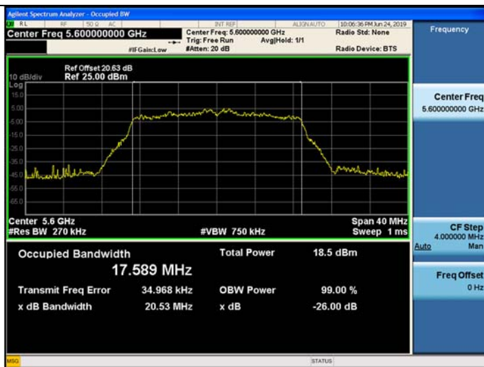
802.11n_HT20 UNII 2C BAND 26dB Bandwidth(CH 120)
