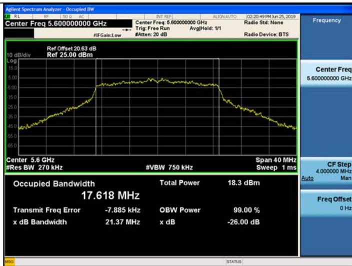
802.11n_HT20 UNII 2C BAND 26dB Bandwidth(CH 120)
