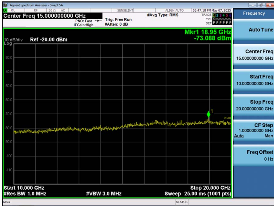
LTE B25_15 M_Conducted Spurious(Above10 G)_Mid_QPSK_1RB
