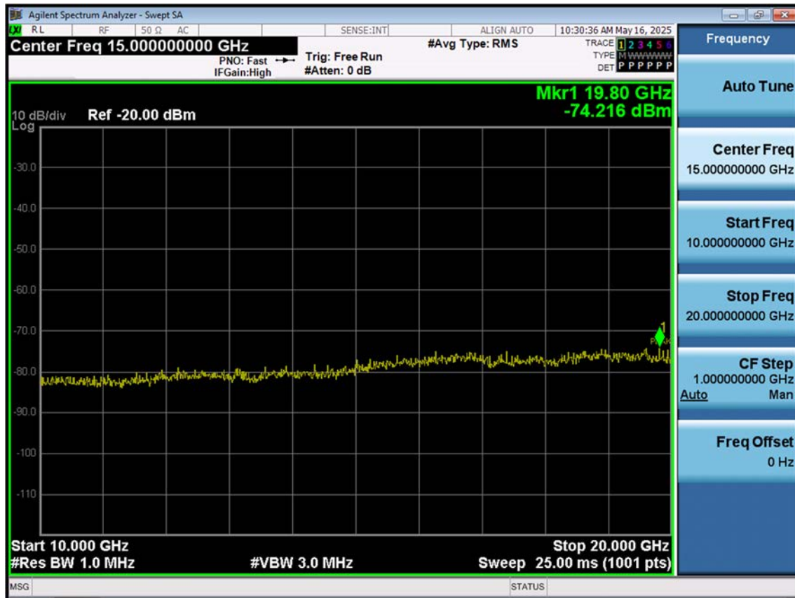
LTE B2_3 M_Conducted Spurious(Above10 G)_Low_QPSK_1RB
