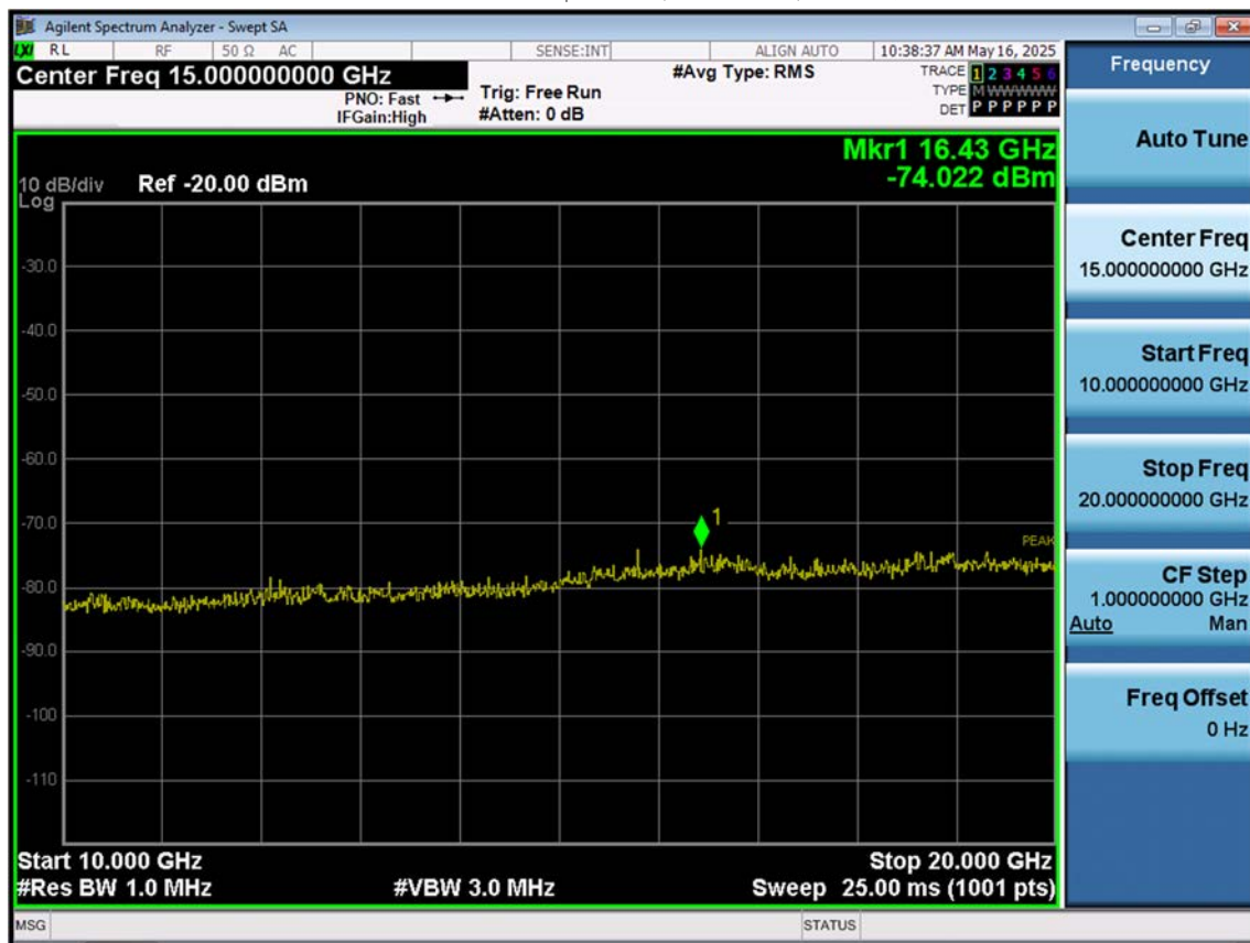
LTE B2_5 M_Conducted Spurious(Above10 G)_Mid_QPSK_1RB
