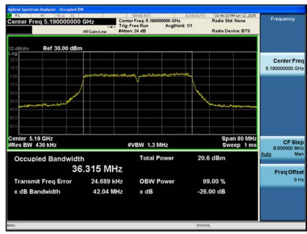
Bandwidth 40M, 802.11ac(VHT40) Ch.38
