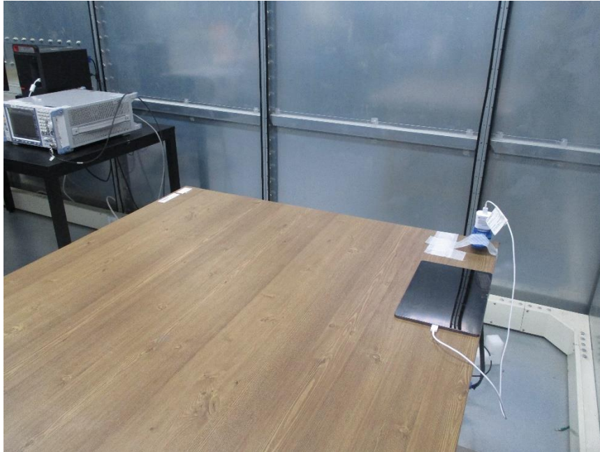
AC LINE CONDUCTED REAR TEST PHOTO
