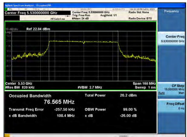
802.11ac(VHT80) 26 dB Bandwidth (CH 106)
