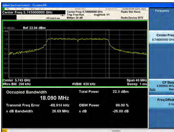
802.11ac(VHT40) 26 dB Bandwidth (CH 149)
