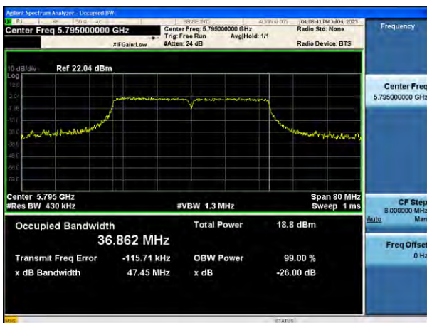
802.11ac(VHT40) 26 dB Bandwidth (CH 149)
