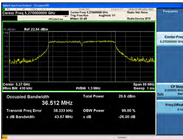
802.11ac(VHT40) 26 dB Bandwidth (CH 54)
