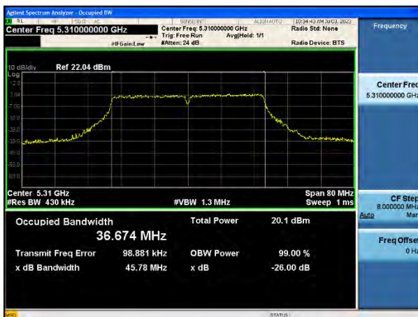
802.11ac(VHT40) 26 dB Bandwidth (CH 62)
