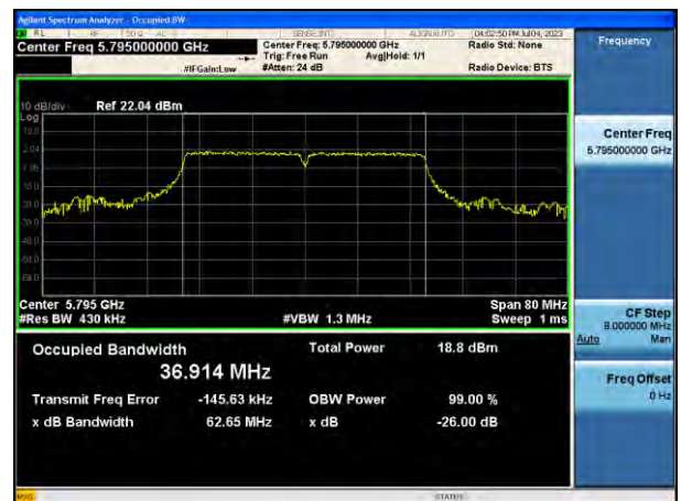
802.11ac(VHT80) 26 dB Bandwidth (CH 106)
