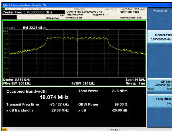
802.11ac(VHT40) 26 dB Bandwidth (CH 62)
