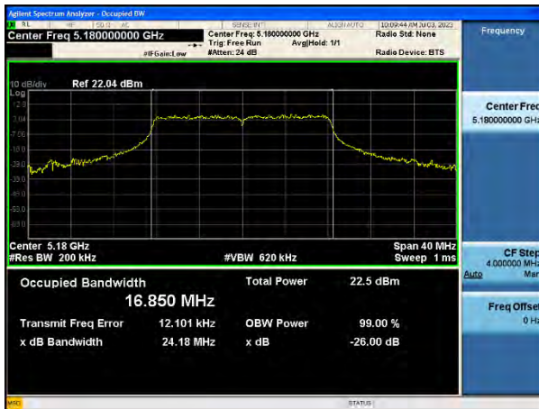
802.11ac(VHT20) 26 dB Bandwidth (CH 157)
