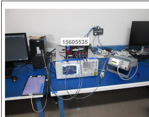
RF ANTENNA PORT CONDUCTED
