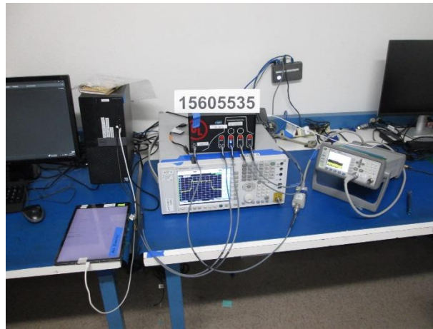
RF ANTENNA PORT CONDUCTED
