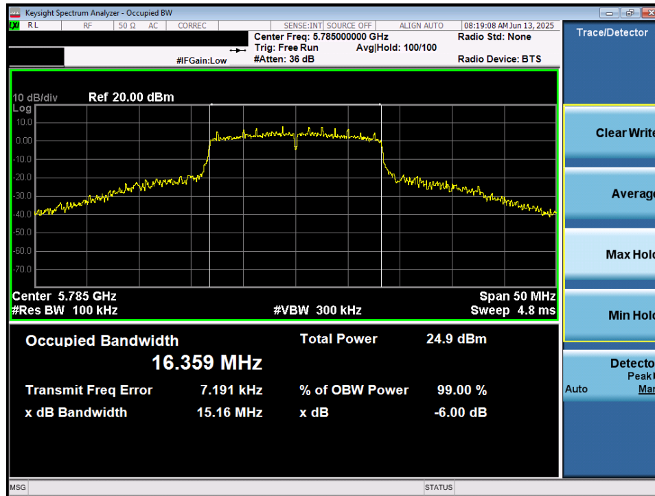
Plot 7-19. 6dB Bandwidth Plot MIMO ANT1 (802.11a (UNII Band 3) – Ch. 157)
