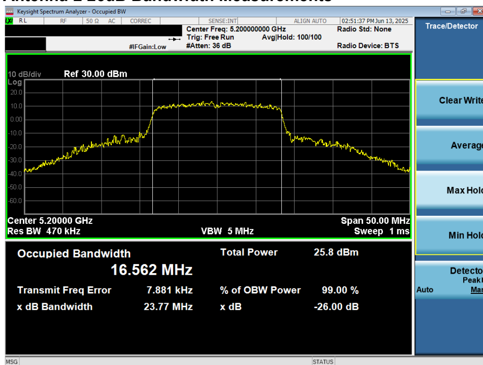
Plot 7-10. 26dB Bandwidth Plot MIMO ANT2 (802.11a (UNII Band 1) – Ch. 40)
