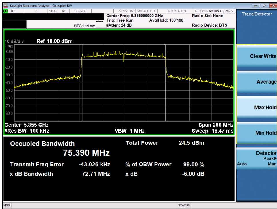
Plot 7-31. 6dB Bandwidth Plot MIMO ANT1 (80MHz BW 802.11ac (UNII Band 3/4) – Ch. 171)
