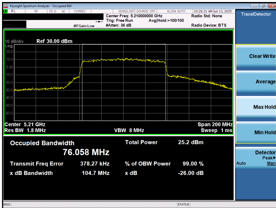
Plot 7-6. 26dB Bandwidth Plot MIMO ANT1 (80MHz BW 802.11ac (UNII Band 1) – Ch. 42)
