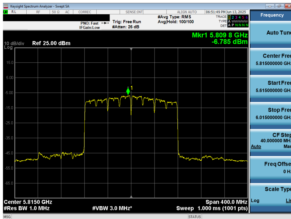
Plot 7-100. Power Spectral Density Plot MIMO ANT2 (160MHz BW 802.11ax (UNII Band 3/4) – Ch. 163)
