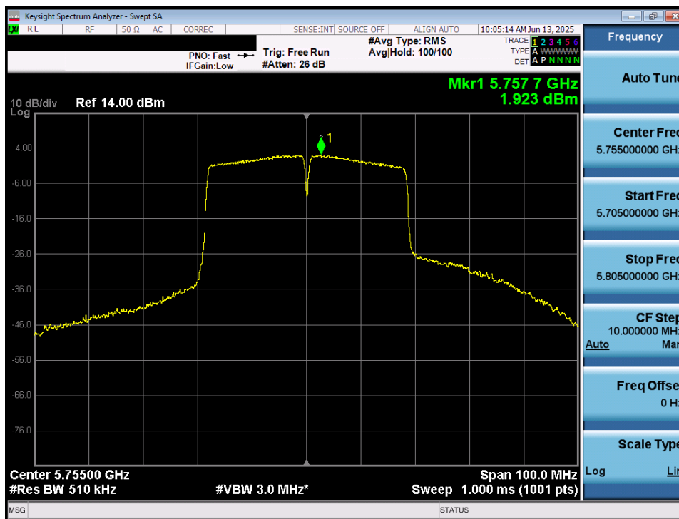
Plot 7-63. Power Spectral Density Plot MIMO ANT1 (40MHz BW 802.11n (UNII Band 3) – Ch. 151)
