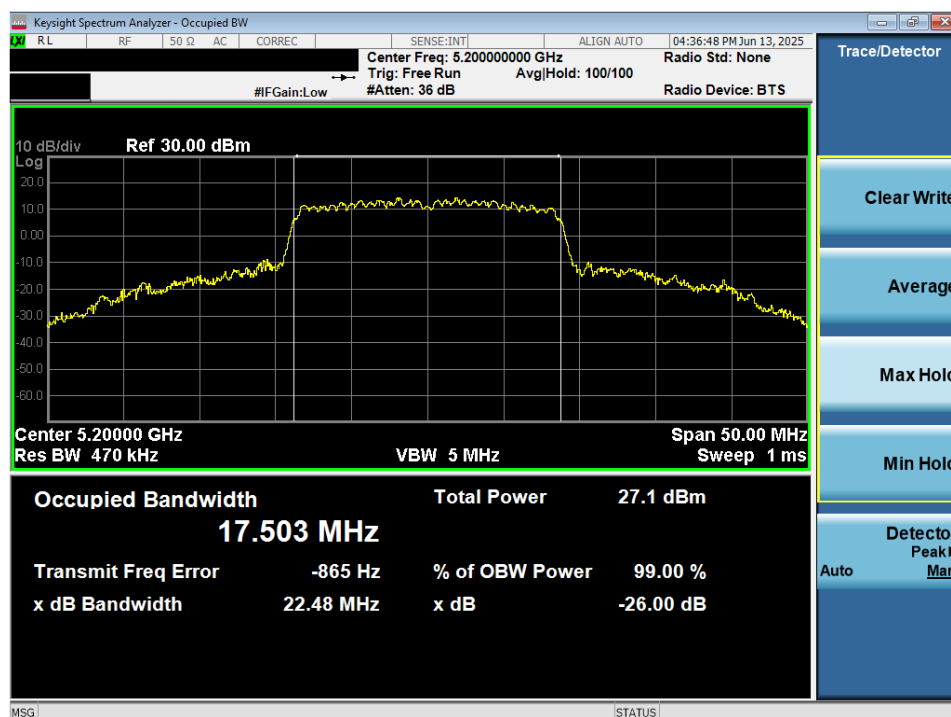
Plot 7-11. 26dB Bandwidth Plot MIMO ANT2 (20MHz BW 802.11n (UNII Band 1) – Ch. 40)
