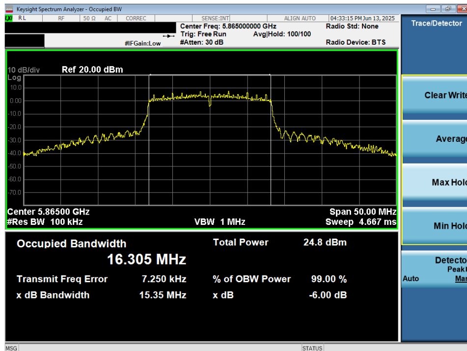
Plot 7-42. 6dB Bandwidth Plot MIMO ANT2 (802.11a (UNII Band 3/4) – Ch. 173)
