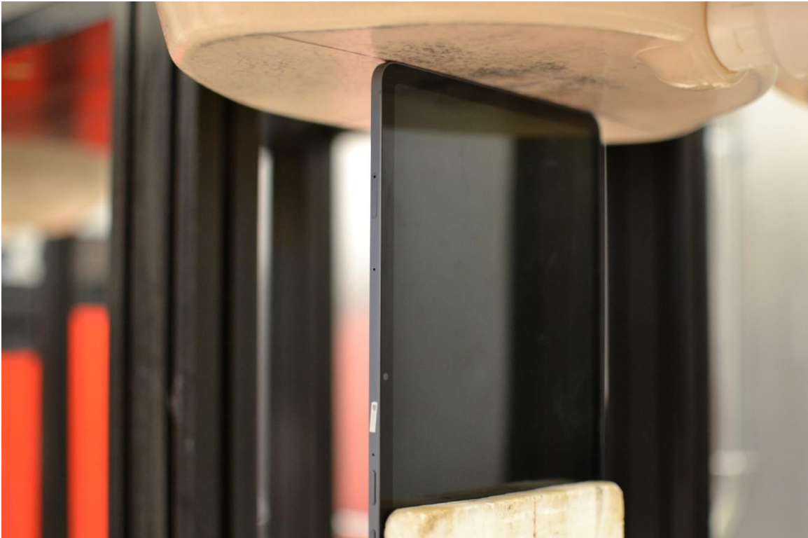
SAR Test Setup Photo 8 – Body, Bottom Edge at 0mm
