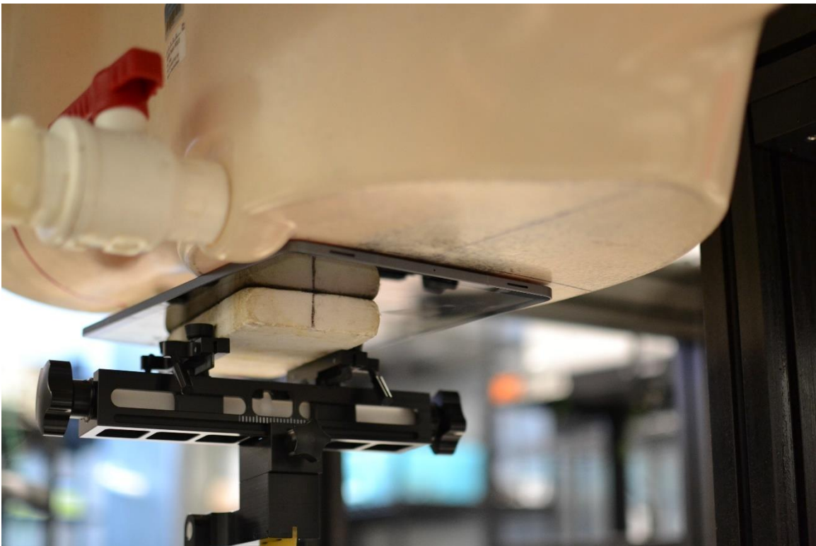
SAR Test Setup Photo 2 – Body, Back Side at 0mm – Antenna WIFI 0
