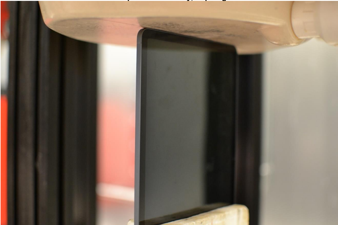
SAR Test Setup Photo 6 – Body, Top Edge at 0mm
