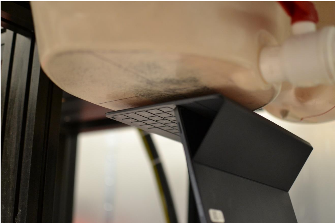
SAR Test Setup Photo 16 – Laptop, Bottom Edge at 11mm
