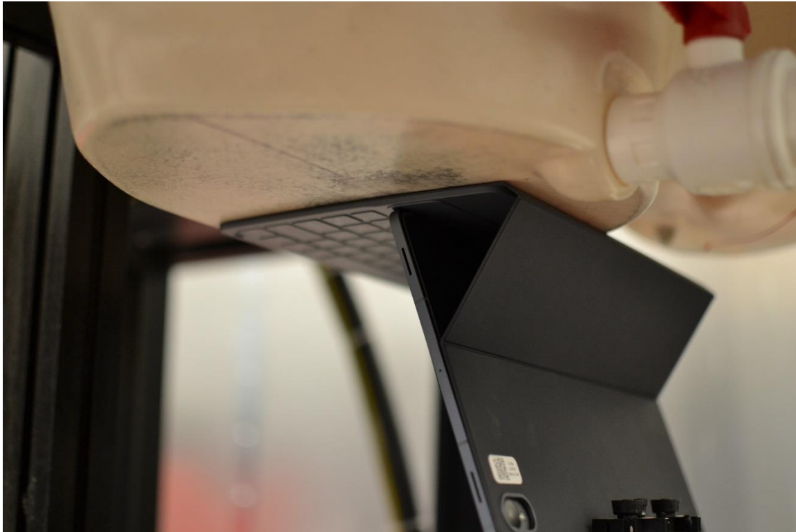
SAR Test Setup Photo 17 – Laptop, Bottom Edge at 0mm
