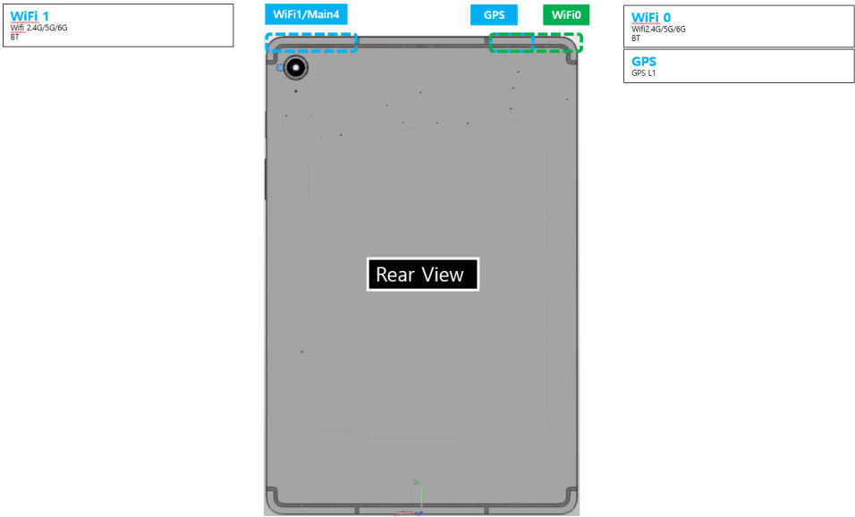
Figure I-1 DUT Antenna Locations
