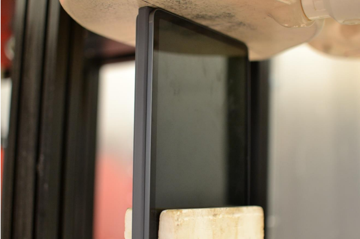
SAR Test Setup Photo 7 – Body with Keyboard, Top Edge at 0mm
