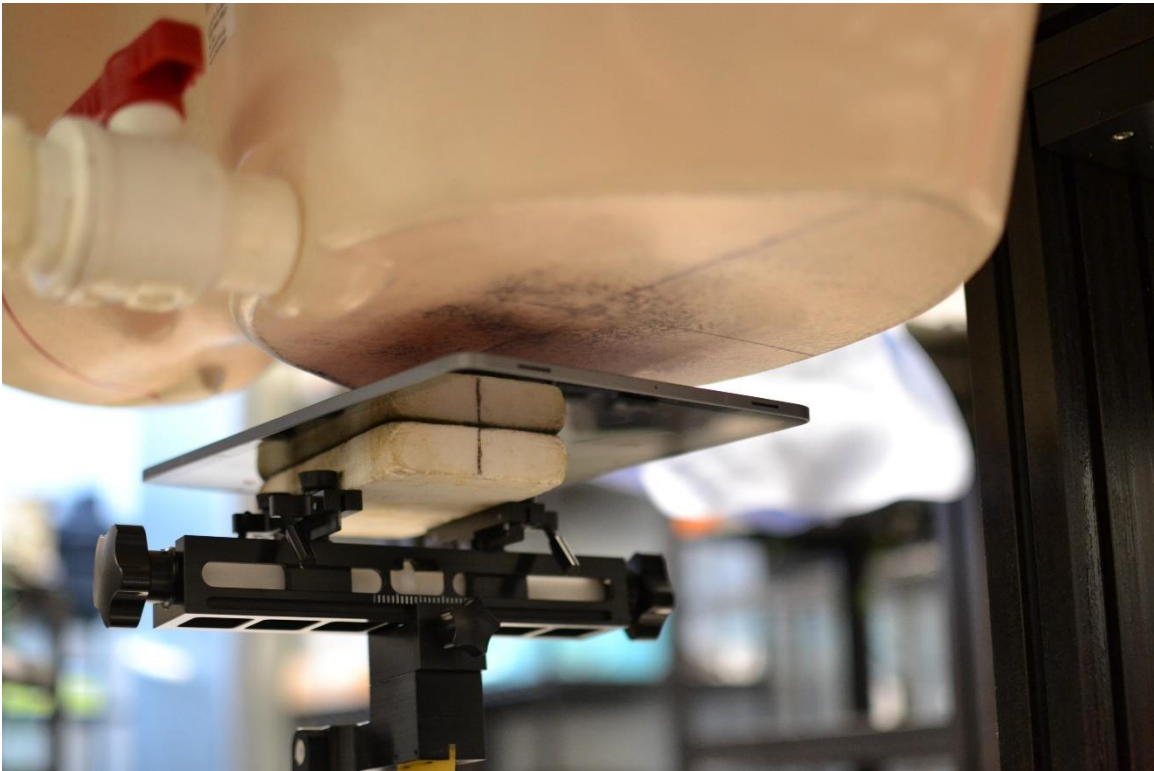
SAR Test Setup Photo 1 – Body, Back Side at 19mm – Antenna WIFI 0
