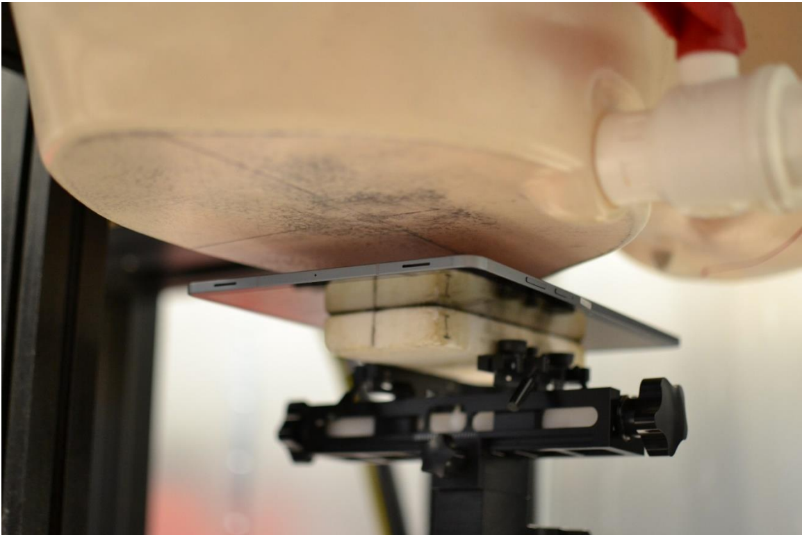
SAR Test Setup Photo 3 – Body, Back Side at 19mm– Antenna WIFI 1
