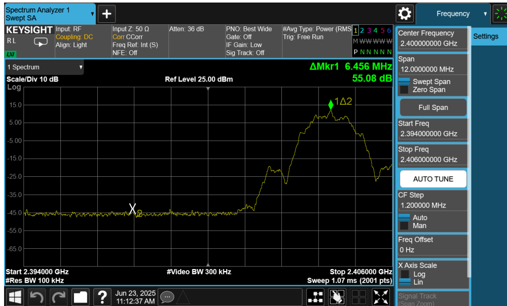
Plot 7-87. Band Edge Plot (Bluetooth (LE), 2Mbps – Ch. 0) – Ant 2
