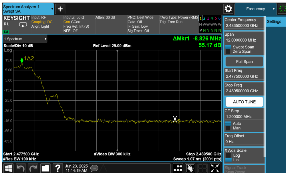
Plot 7-88. Band Edge Plot (Bluetooth (LE), 2Mbps – Ch. 36) – Ant 2
