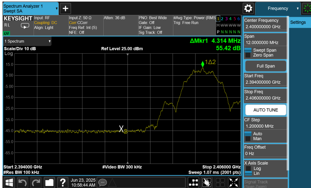
Plot 7-79. Band Edge Plot (Bluetooth (LE), 2Mbps – Ch. 0) – Ant 1
