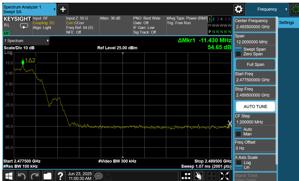
Plot 7-80. Band Edge Plot (Bluetooth (LE), 2Mbps – Ch. 36) – Ant 1
