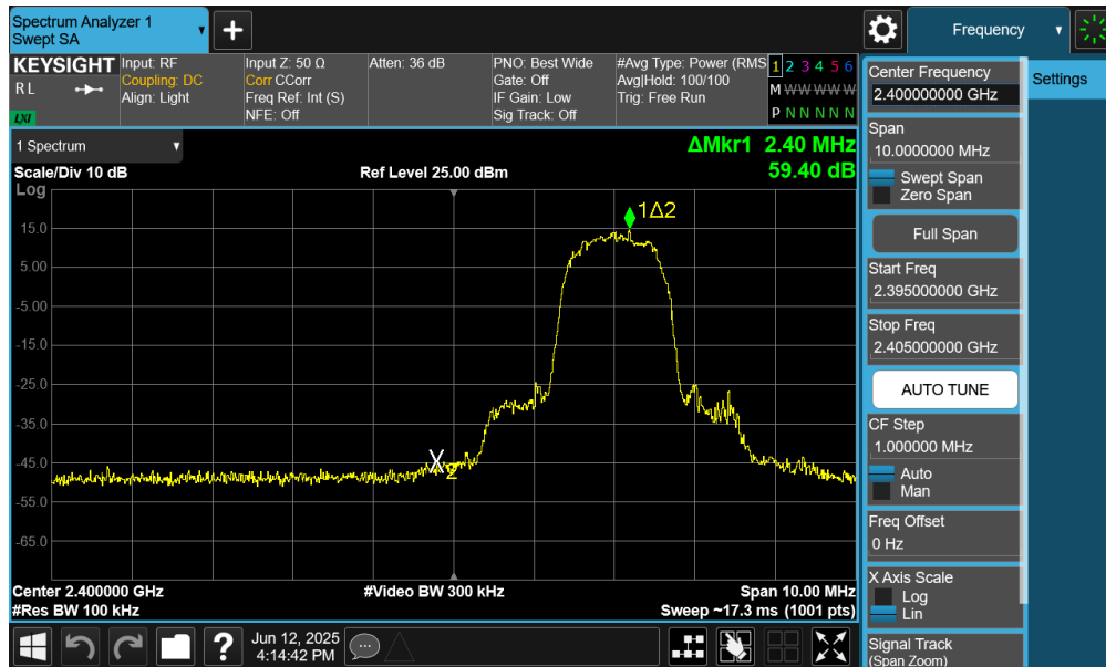
Plot 7-55. Band Edge Plot (Bluetooth with Hopping Disabled, 3 Mbps – Ch. 0) – ANT1
