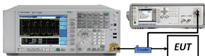
Figure 7-7. Test Instrument & Measurement Setup
