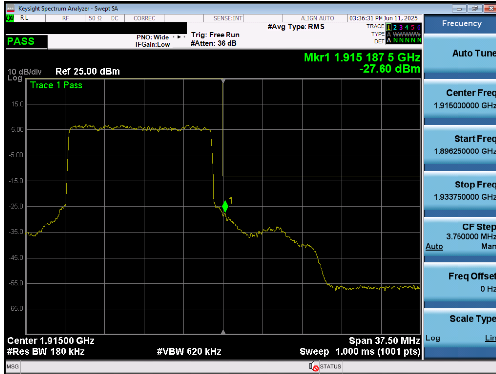
Plot 7-110. Upper Band Edge Plot (NR Band n25 - 15MHz QPSK - Full RB)
