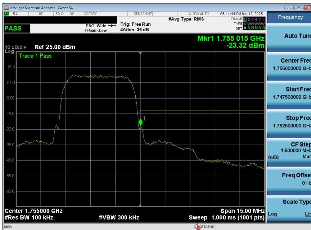
Plot 7-79. Upper Band Edge Plot (WCDMA AWS – Ch. 1513 – ANT1)
