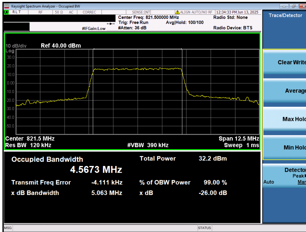
Plot 7-5. Occupied Bandwidth Plot (LTE Band 26 - 5MHz QPSK - Full RB)
