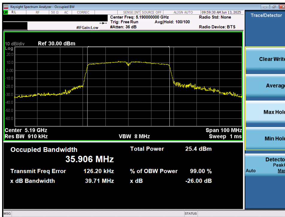
Plot 7-4. 26dB Bandwidth Plot MIMO ANT1 (40MHz BW 802.11n (UNII Band 1) – Ch. 38)
