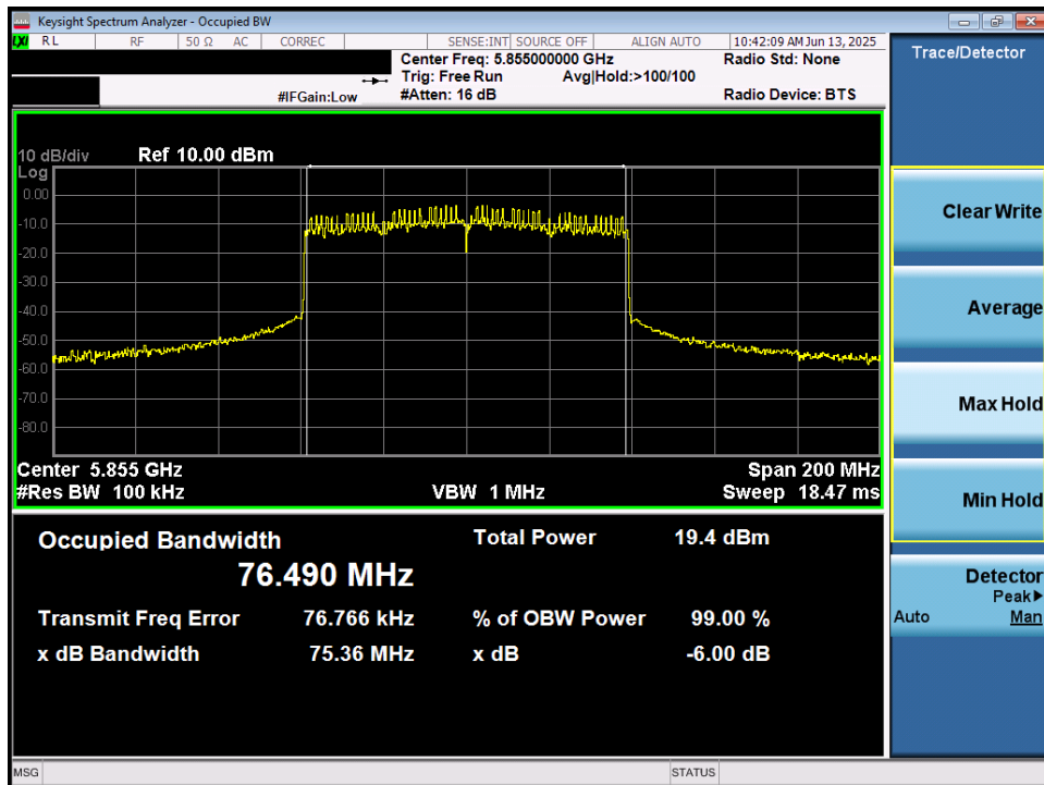
Plot 7-32. 6dB Bandwidth Plot MIMO ANT1 (80MHz BW 802.11ax (UNII Band 3/4) – Ch. 171)
