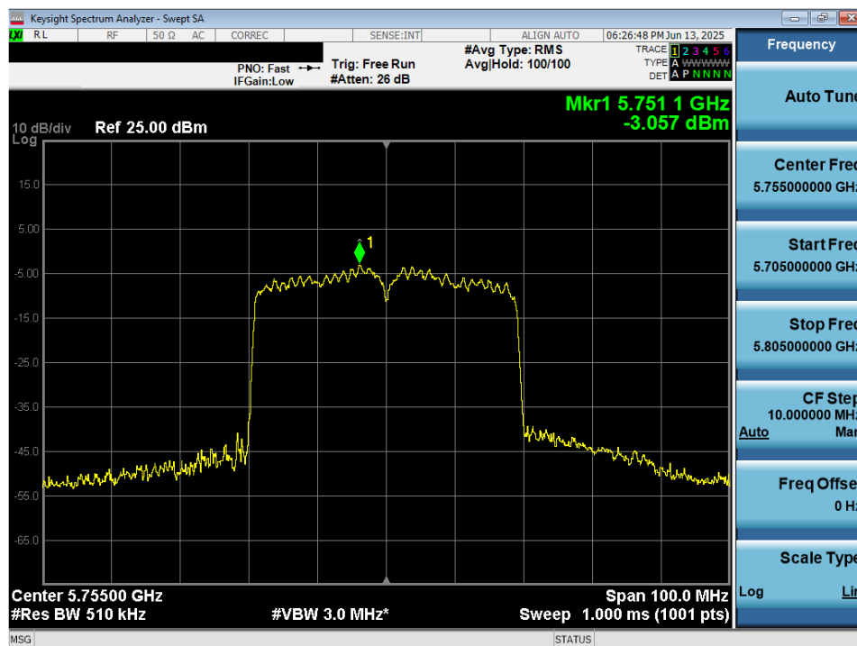
Plot 7-89. Power Spectral Density Plot MIMO ANT2 (40MHz BW 802.11ax (UNII Band 3) – Ch. 151)
