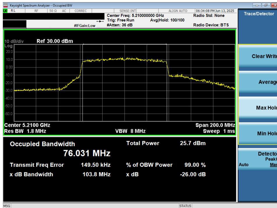
Plot 7-15. 26dB Bandwidth Plot MIMO ANT2 (80MHz BW 802.11ac (UNII Band 1) – Ch. 42)
