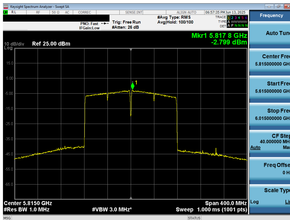
Plot 7-99. Power Spectral Density Plot MIMO ANT2 (160MHz BW 802.11ac (UNII Band 3/4) – Ch. 163)
