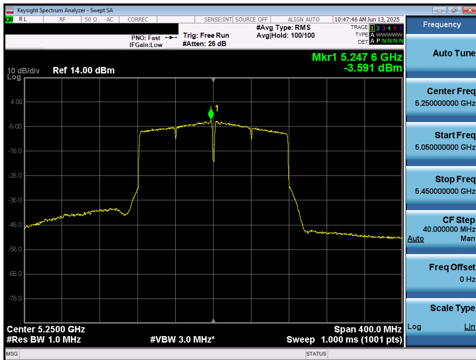
Plot 7-58. Power Spectral Density Plot MIMO ANT1 (160MHz BW 802.11ac (UNII Band 1/2A) – Ch. 50)
