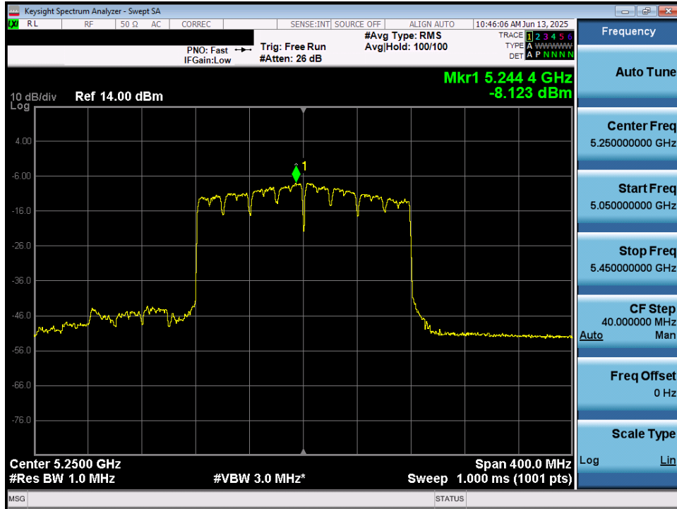
Plot 7-59. Power Spectral Density Plot MIMO ANT1 (160MHz BW 802.11ax (UNII Band 1/2A) – Ch. 50)
