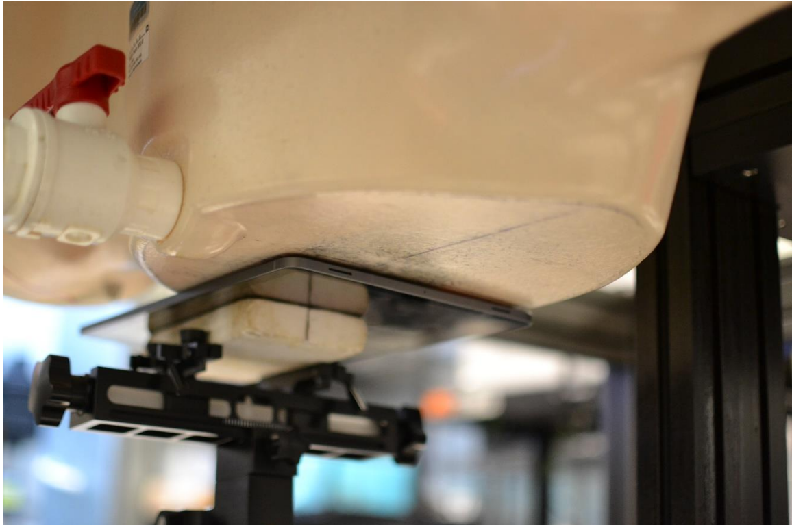
SAR Test Setup Photo 4 – Body, Back Side at 0mm – Antenna WIFI 0
