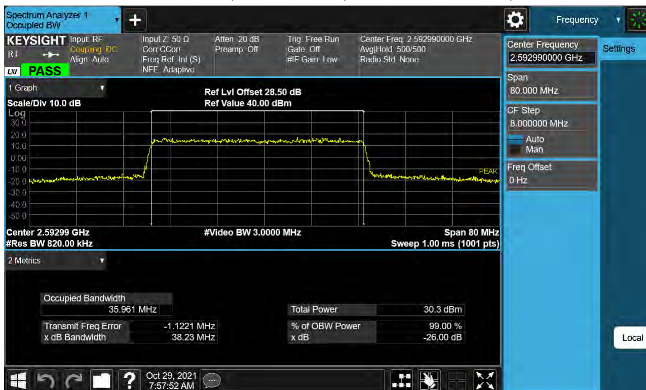
Sub6 n41. Occupied Bandwidth Plot (40 MHz Ch.518598 256-QAM )
