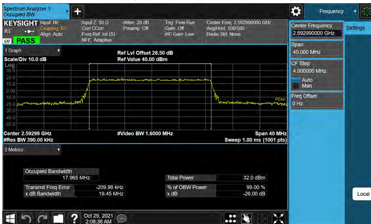
Sub6 n41. Occupied Bandwidth Plot (20 MHz Ch.518598 16-QAM )
