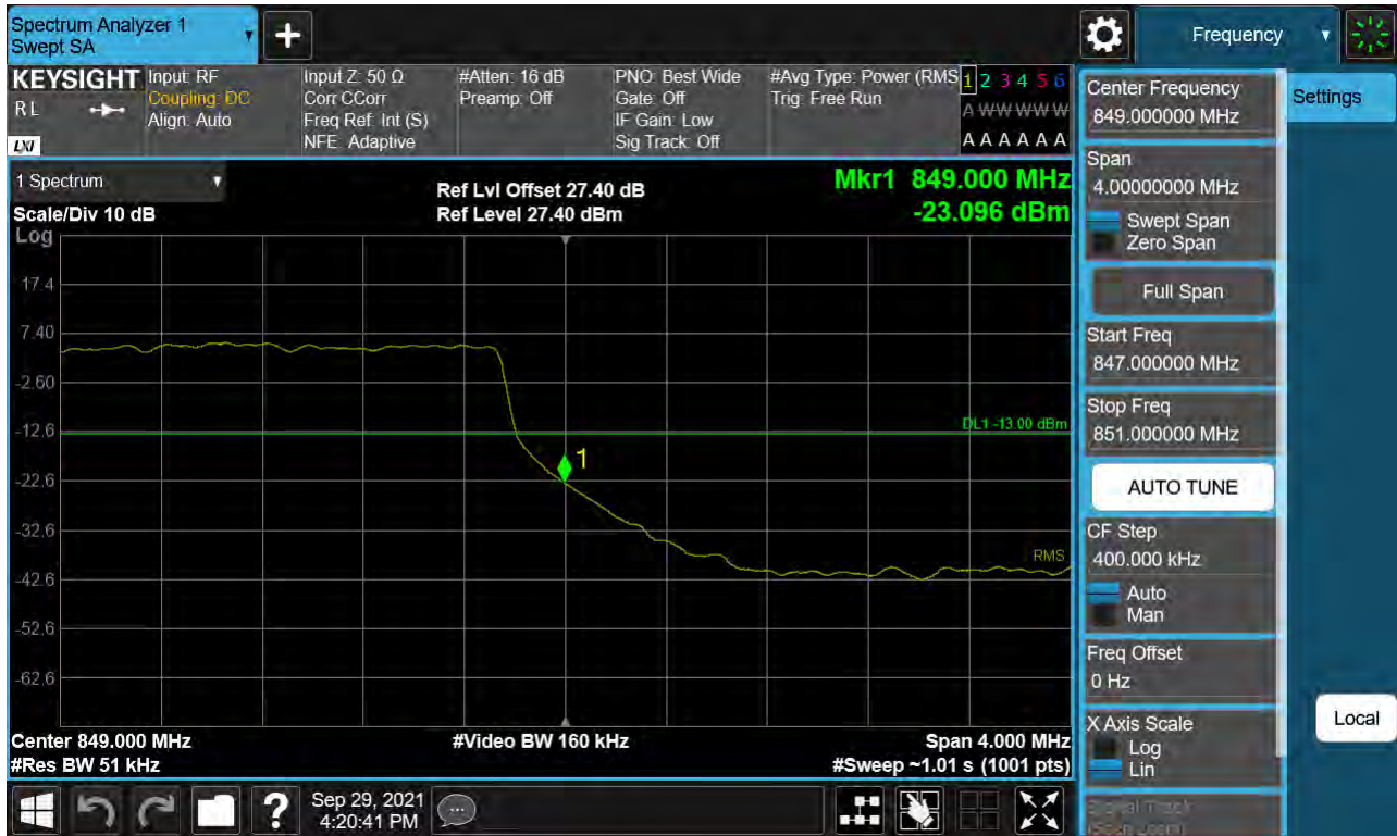
Sub6 n5. Upper Band Edge Plot (5 M BW Ch.169300 BPSK_RB25_Offset 0)
