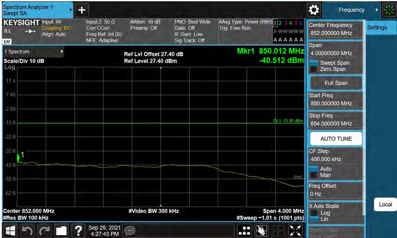
Sub6 n5. Upper Extended Band Edge Plot (10 M BW Ch.168800 BPSK_RB50_0)
