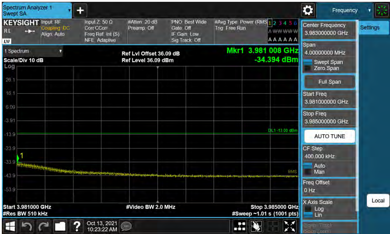
Sub6 n77. High Band Edge Plot (100 M BW Ch.662000 BPSK 1RB)(2)
