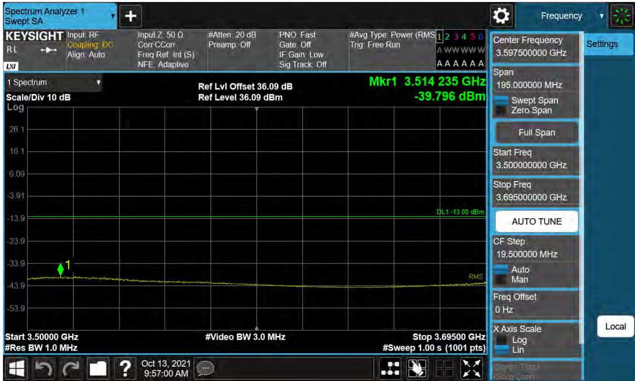
Sub6 n77. Low Band Edge Plot (90 M BW Ch.649668 BPSK 1RB)(3)
