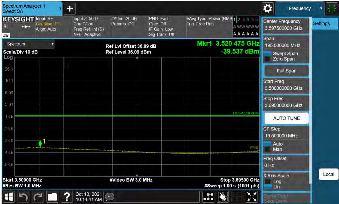
Sub6 n77. Low Band Edge Plot (100 M BW Ch.650000 BPSK 1RB)(3)
