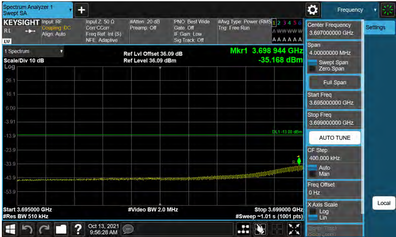
Sub6 n77. Low Band Edge Plot (90 M BW Ch.649668 BPSK 1RB)(2)
