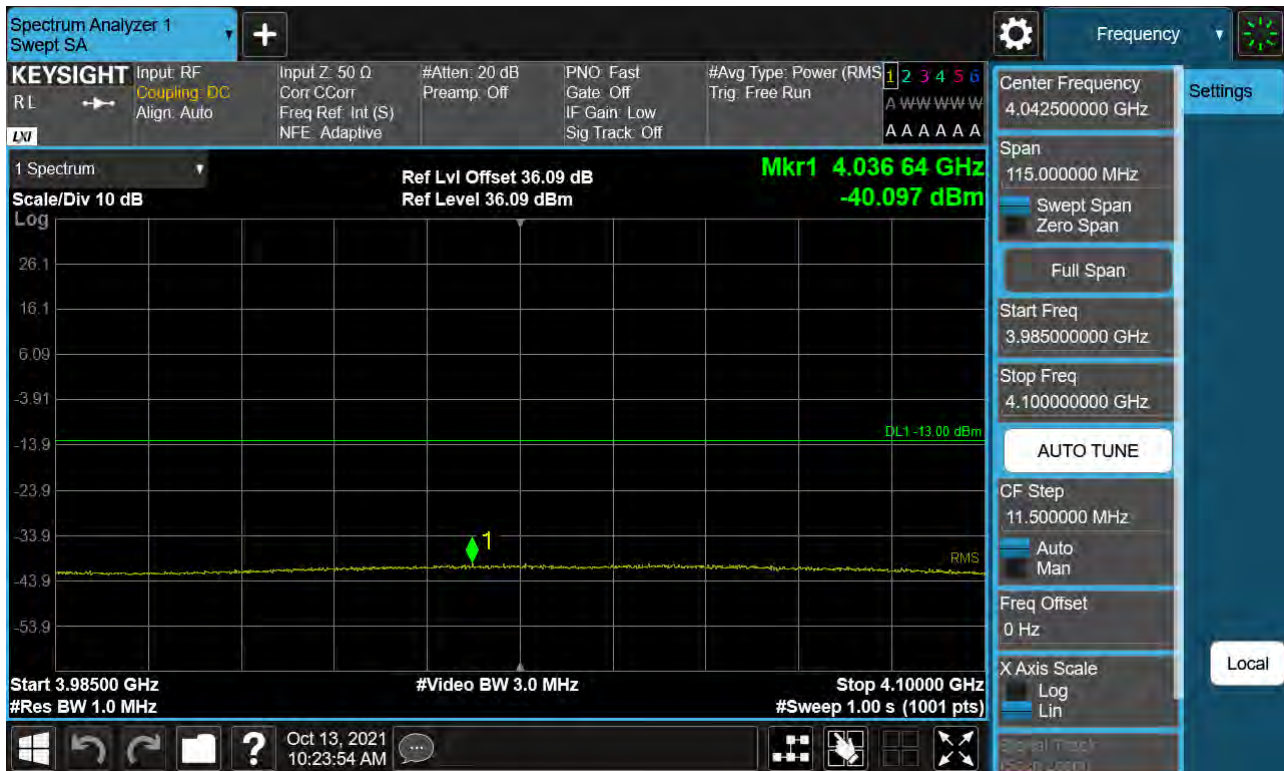
Sub6 n77. High Band Edge Plot (100 M BW Ch.662000 BPSK 1RB)(3)
