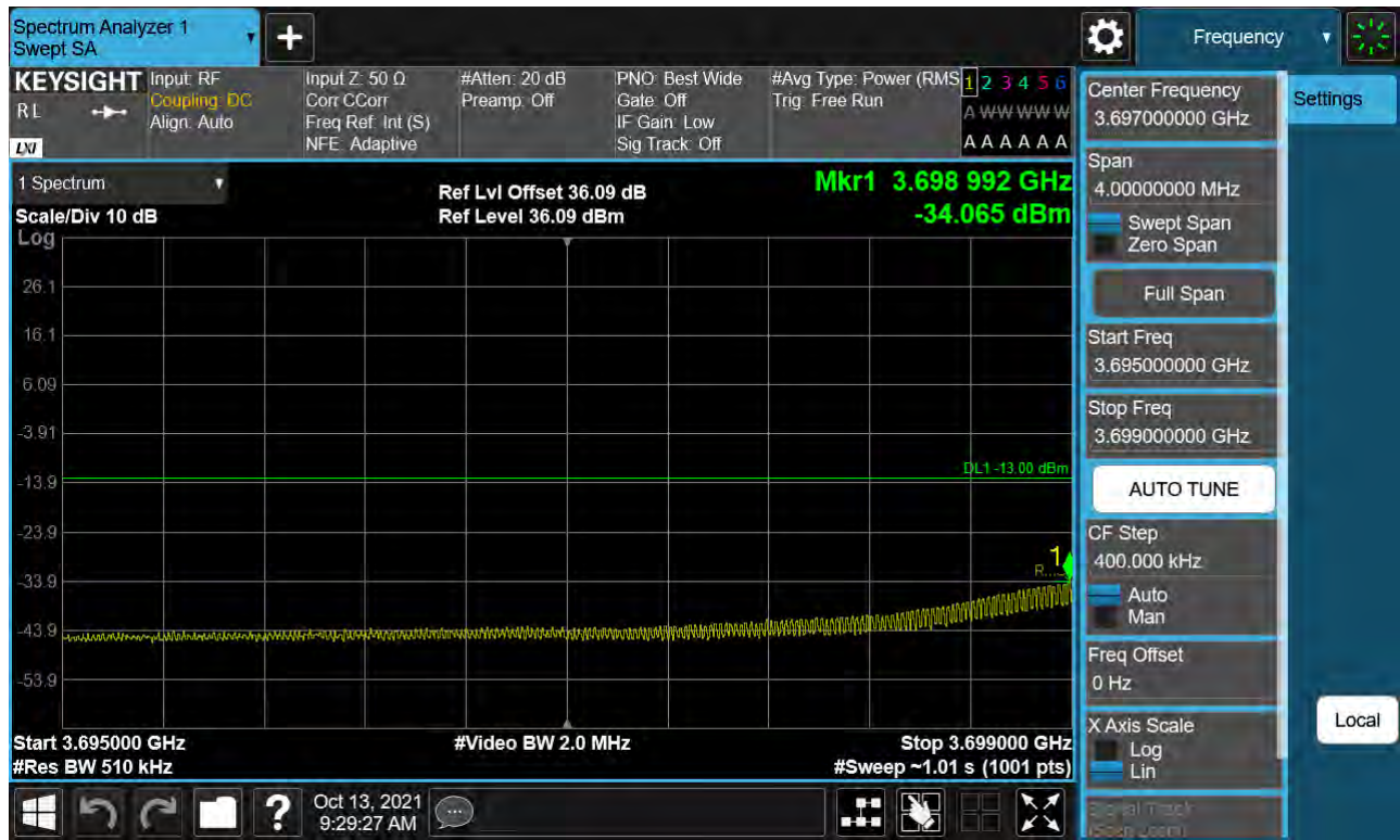
Sub6 n77. Low Band Edge Plot (70 M BW Ch.649000 BPSK 1RB)(2)
