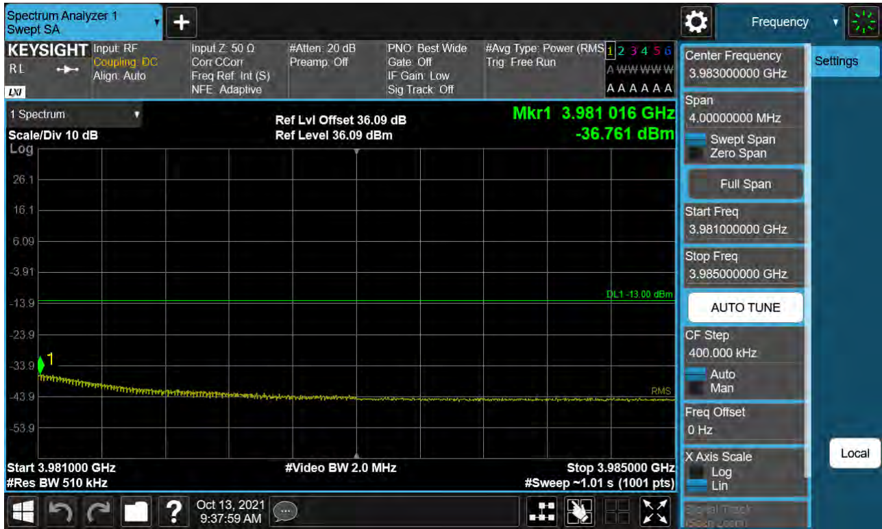
Sub6 n77. High Band Edge Plot (70 M BW Ch.663000 BPSK 1RB)(2)
