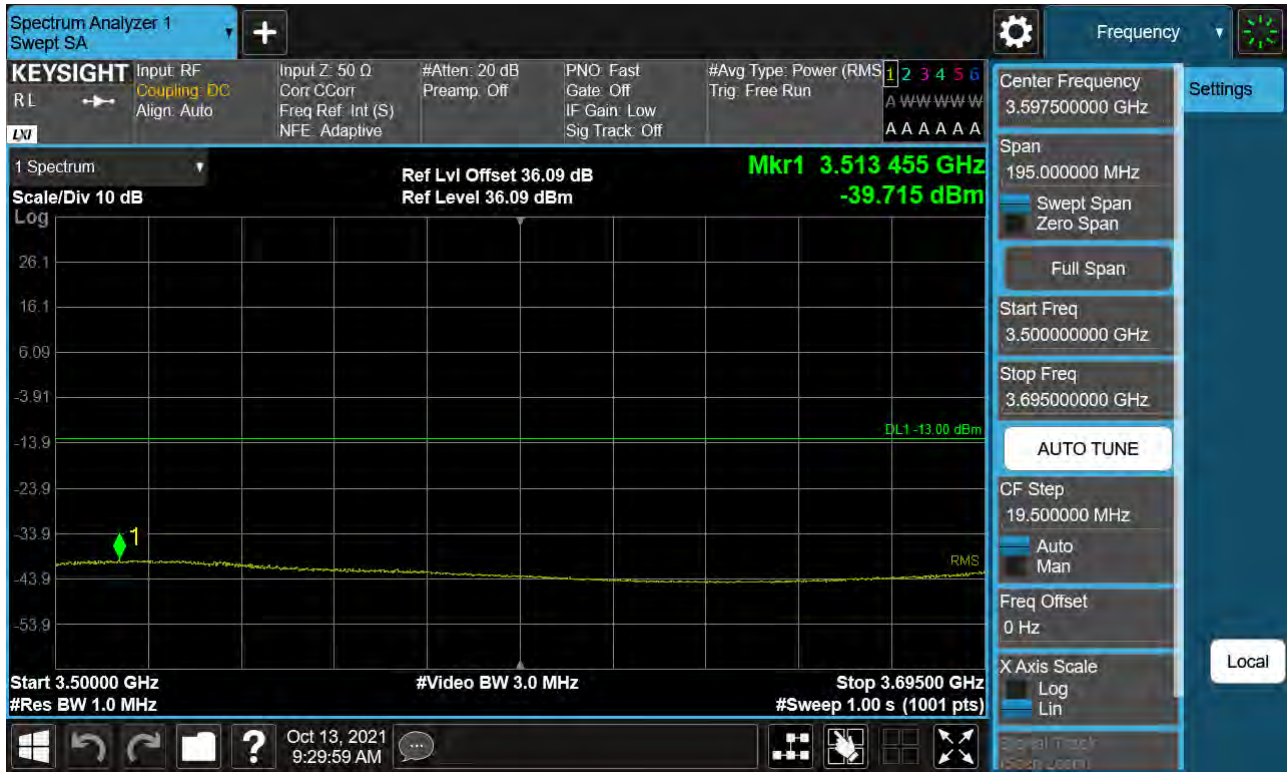
Sub6 n77. Low Band Edge Plot (70 M BW Ch.649000 BPSK 1RB)(3)
