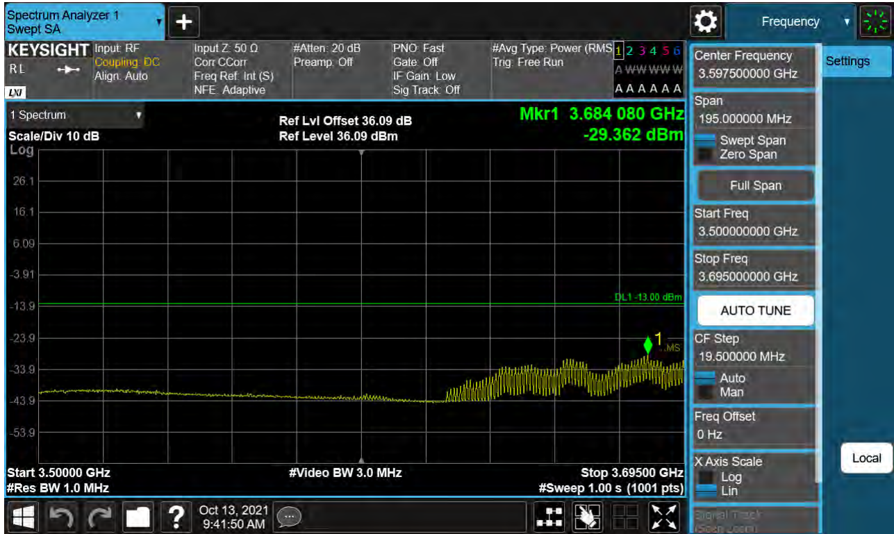
Sub6 n77. Low Band Edge Plot (80 M BW Ch.649334 BPSK FullRB)(3)
