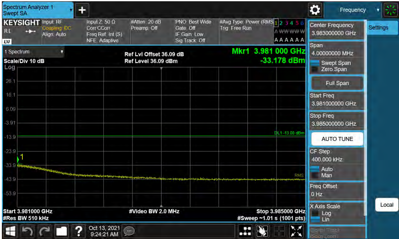
Sub6 n77. High Band Edge Plot (60 M BW Ch.663332 BPSK 1RB)(2)
