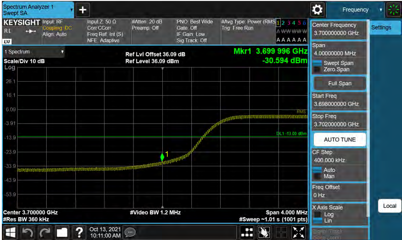
Sub n77. Low Band Edge Plot (100 M BW Ch.650000 BPSK FullRB)(1)
