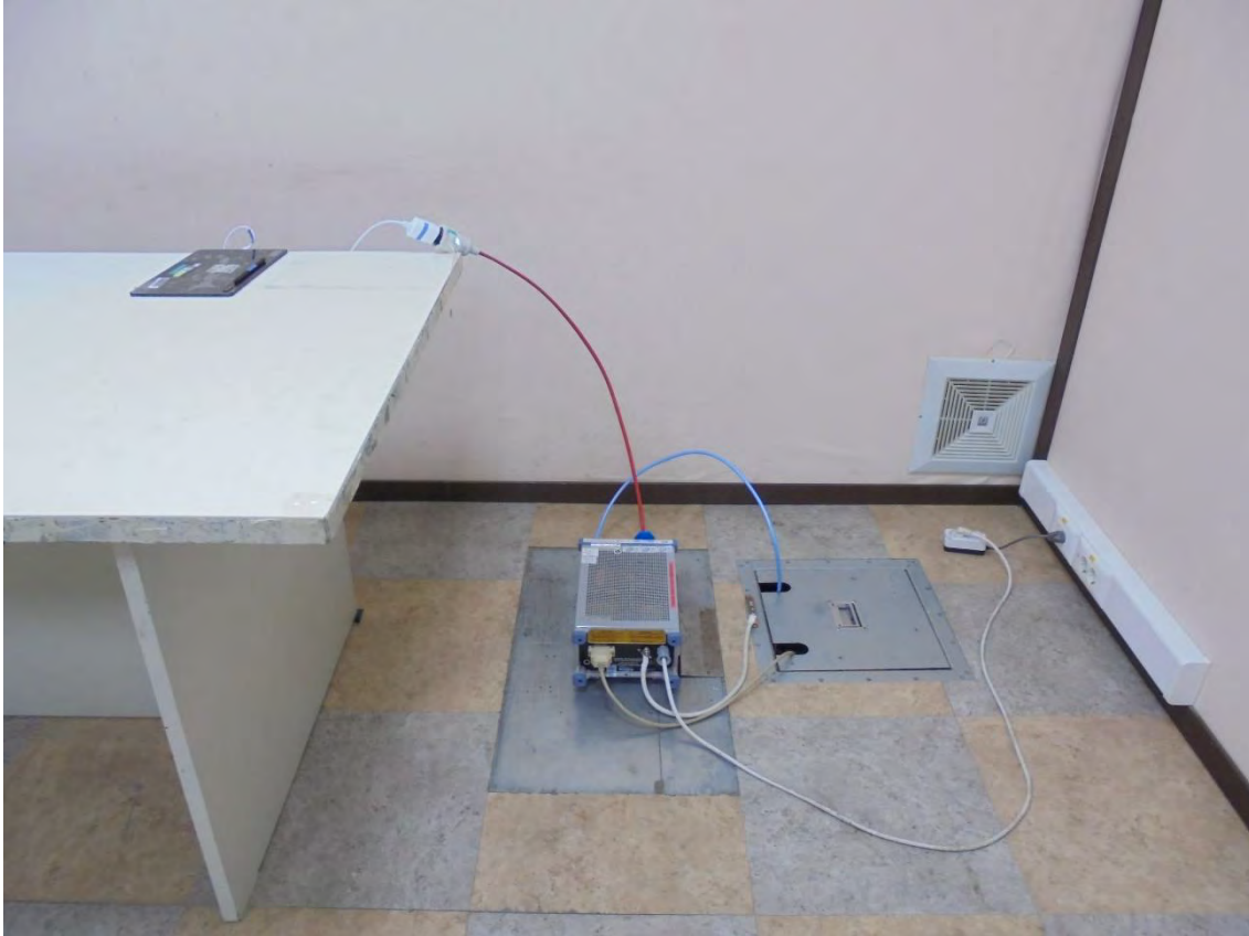
AC Power Line Conducted Test WPS (S-Pen) Setup Photo
