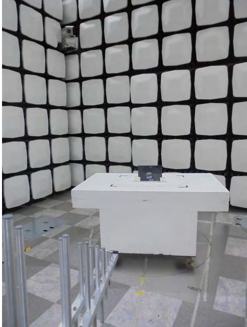
WPT Radiated Test Setup Photo for 30 MHz ~ 1 GHz :
