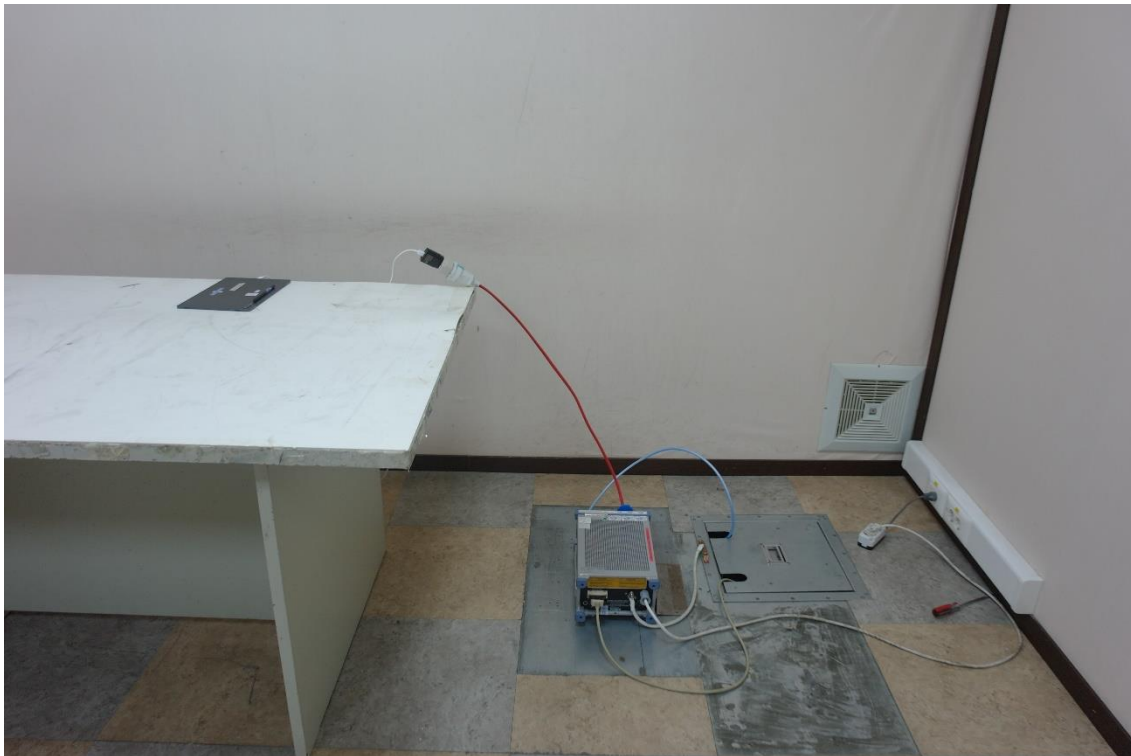
AC PowerLine Conducted Test WPS(S-pen) Setup Photo
