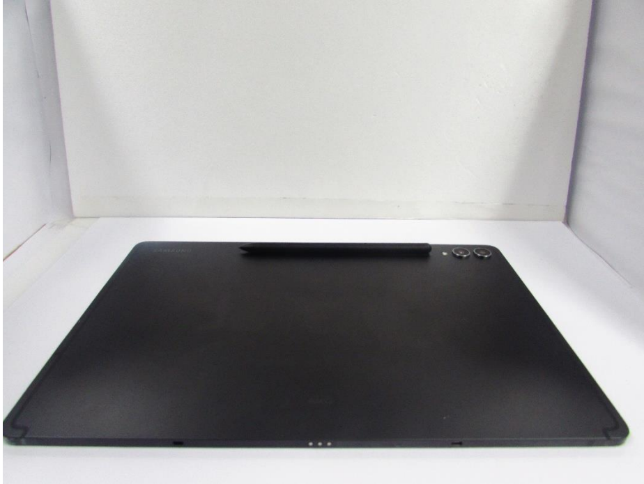
Positions of SPEN and DUT during charging.
