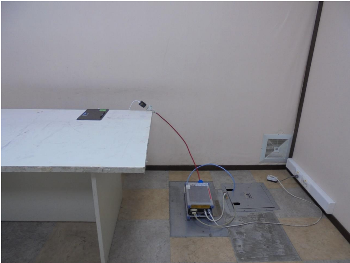
AC PowerLine Conducted Test WPS(S-pen) Setup Photo
