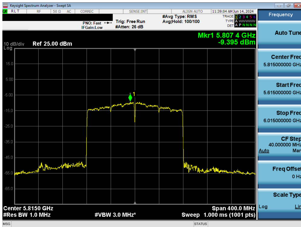
Plot 7-109. Power Spectral Density Plot MIMO ANT1 (160MHz BW 802.11ax – 996*2 Tones (UNII Band 3/4) – Ch. 163)
