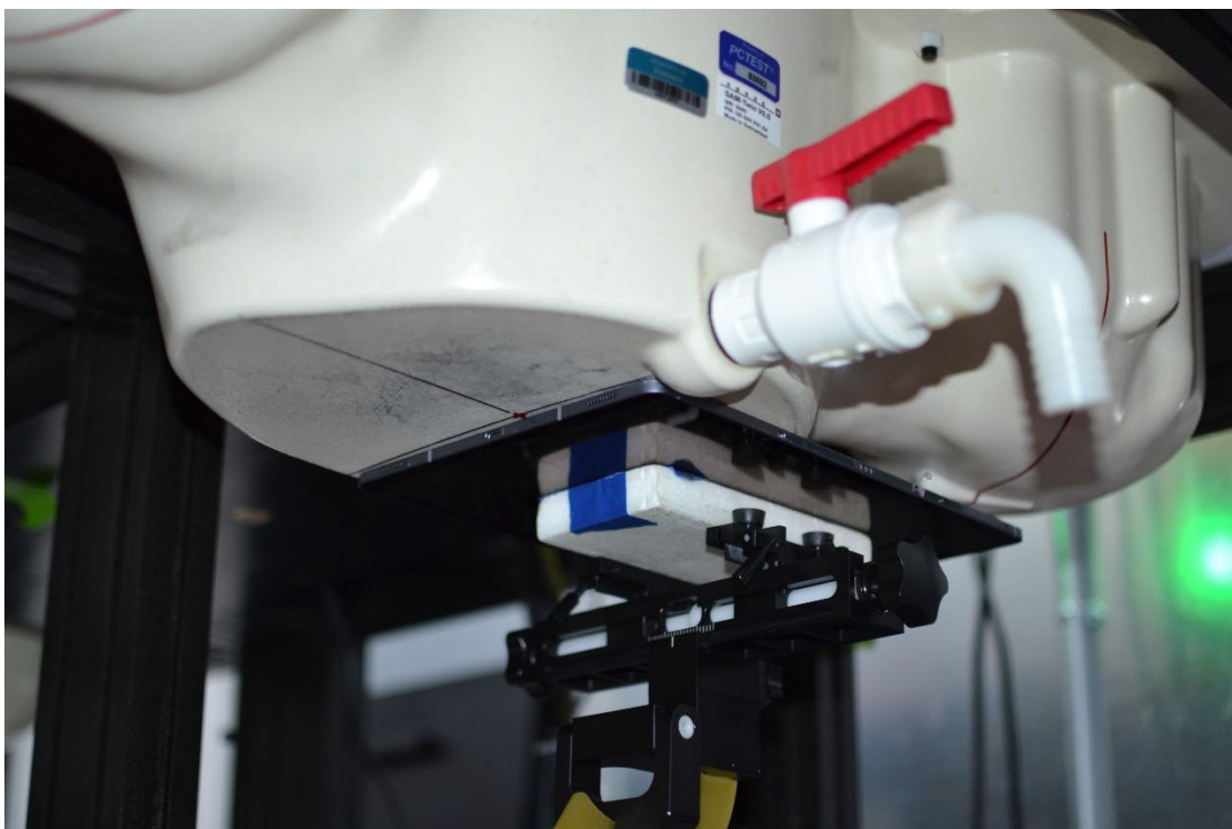
SAR Test Setup Photo 6 – Tablet, Back Side at 0 mm – Antenna M2
