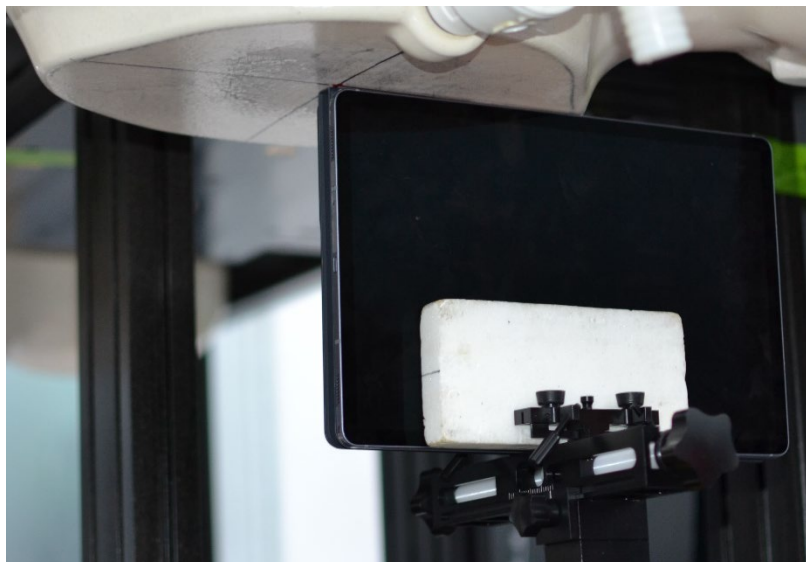
SAR Test Setup Photo 32 – Tablet with Keyboard Variant 2, Left Edge at 0 mm – Antenna S1, S2, S4, or M2
