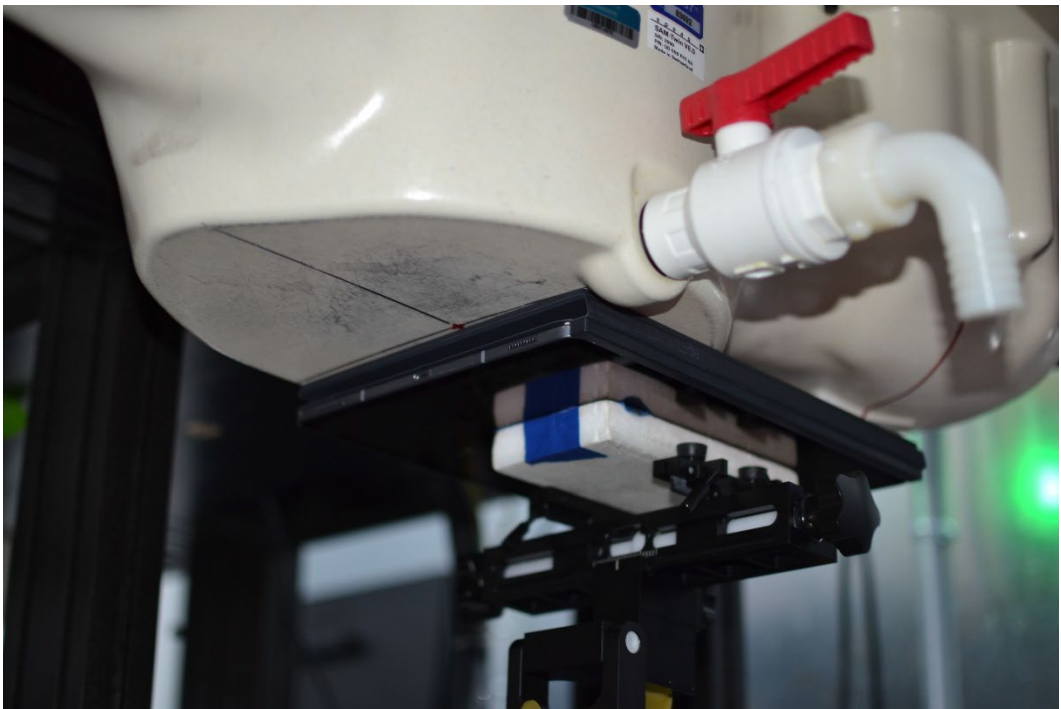
SAR Test Setup Photo 23 – Tablet with Keyboard Variant 1, Back Side at 0 mm – Antenna S2 or S4
