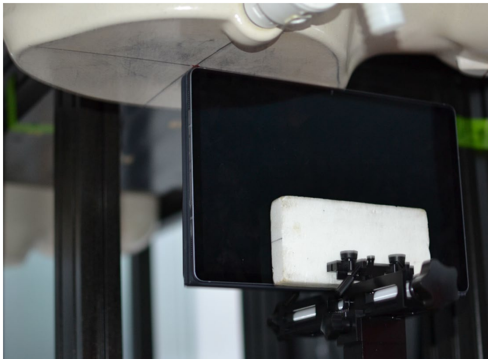
SAR Test Setup Photo 36 – Tablet with Keyboard Variant 2, Right Edge at 0 mm – Antenna WIFI 1, 2, M1, or S3
