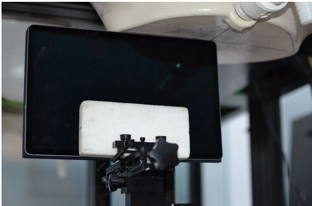
SAR Test Setup Photo 39 – Tablet with Keyboard Variant 2, Right Edge at 0 mm – Antenna S1, S2, S4, or M2
