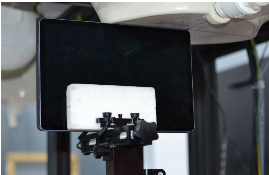
SAR Test Setup Photo 28 – Tablet with Keyboard Variant 1, Left Edge at 0 mm – Antenna WIFI 1, 2, M1, or S3
