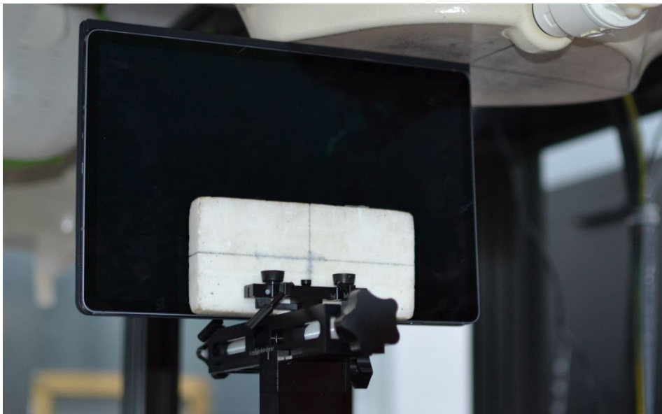
SAR Test Setup Photo 27 – Tablet with Keyboard Variant 1, Left Edge at 0 mm – Antenna WIFI 1, 2, M1, or S3
