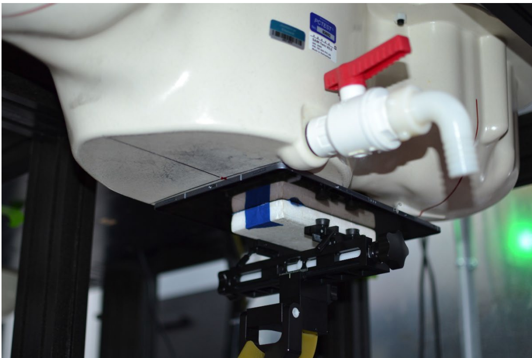
SAR Test Setup Photo 22 – Tablet, Back Side at 0 mm – Antenna S2 or S4
