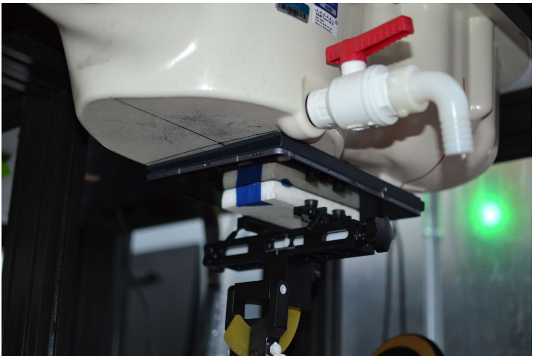
SAR Test Setup Photo 24 – Tablet with Keyboard Variant 2, Back Side at 0 mm – Antenna S2 or S4
