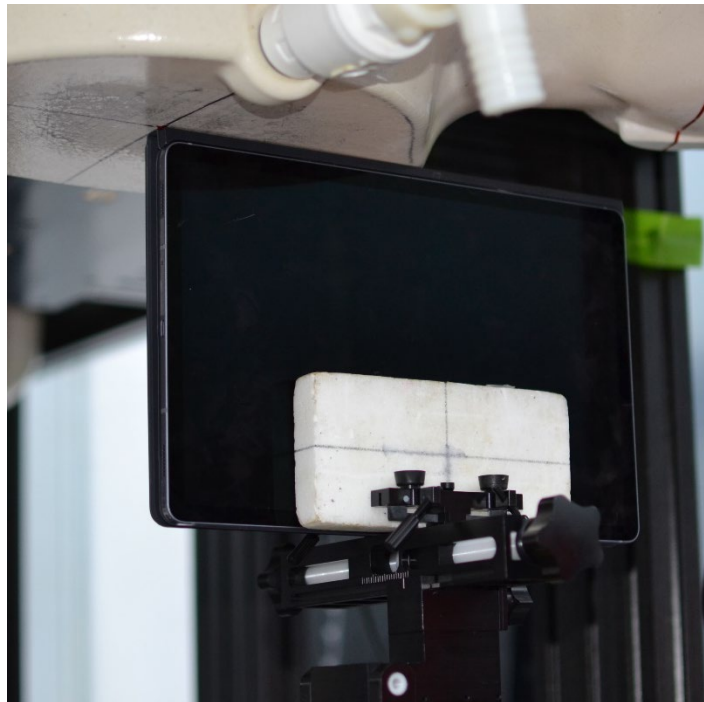
SAR Test Setup Photo 31 – Tablet with Keyboard Variant 1, Left Edge at 0 mm – Antenna S1, S2, S4, or M2
