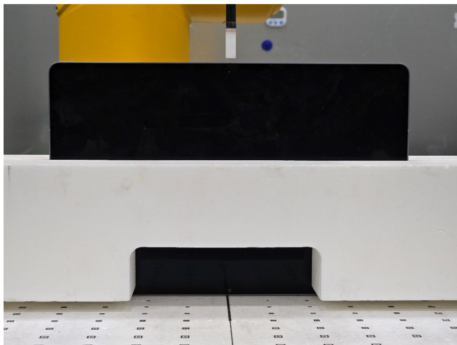
SAR Test Setup Photo 60 – Tablet, Left Edge at 2 mm
