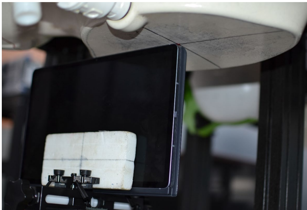
SAR Test Setup Photo 38 – Tablet with Keyboard Variant 1, Right Edge at 0 mm – Antenna S1, S2, S4, or M2
