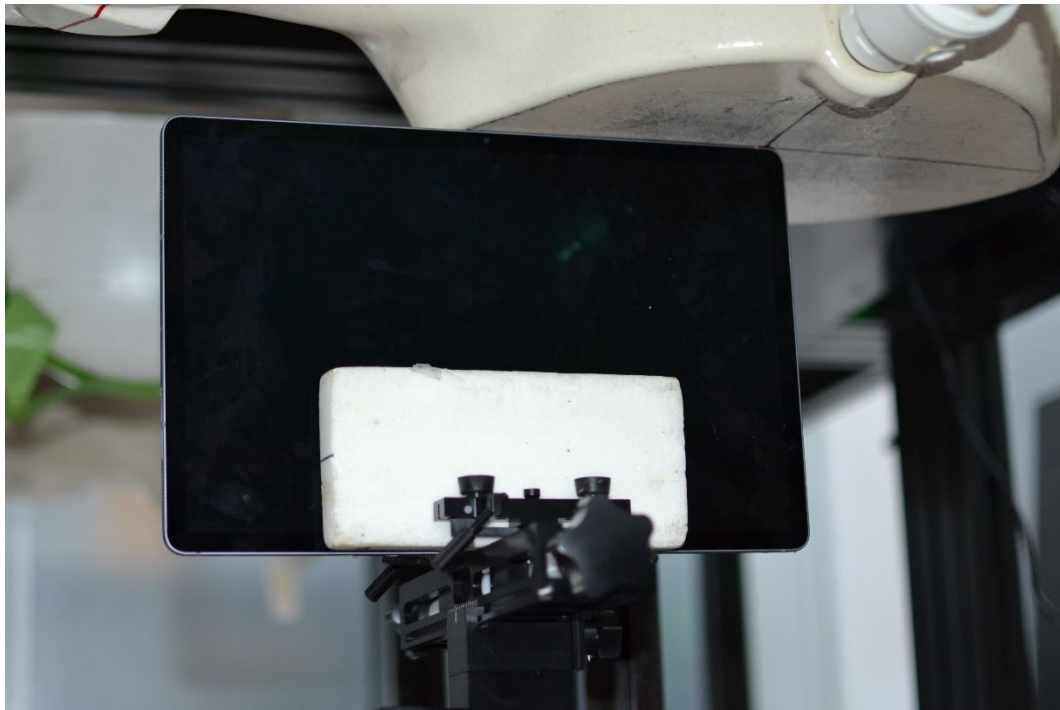
SAR Test Setup Photo 37 – Tablet, Right Edge at 0 mm – Antenna S1, S2, S4, or M2
