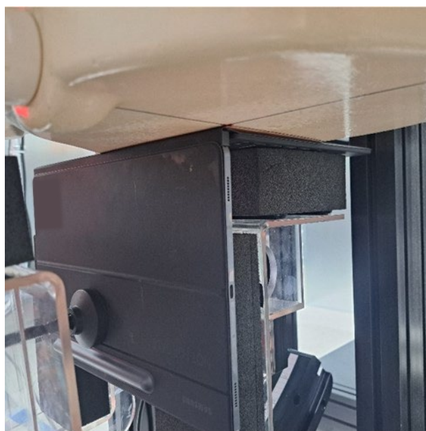
SAR Test Setup Photo 52 – Laptop with Keyboard Variant 1, Bottom Edge at 0 mm Antenna M2, S1, S2, or S4
