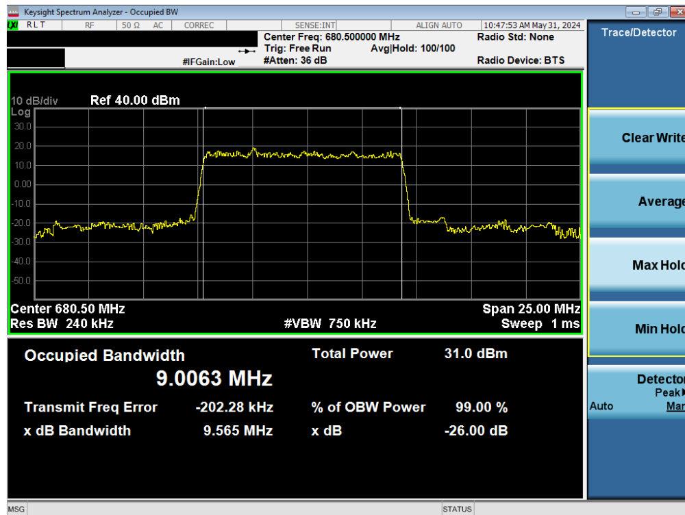
Plot 7-28. Occupied Bandwidth Plot (NR Band n71 - 10MHz DFT-s-OFDM BPSK - Full RB – ANT1)
