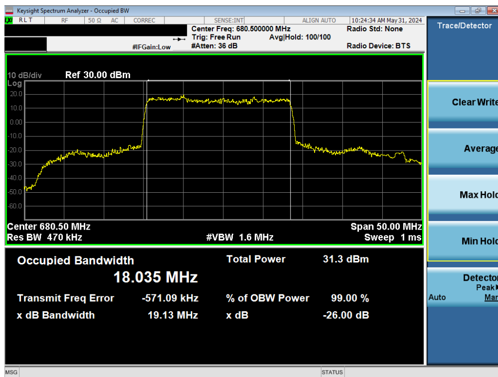
Plot 7-22. Occupied Bandwidth Plot (NR Band n71 - 20MHz DFT-s-OFDM BPSK - Full RB – ANT1)
