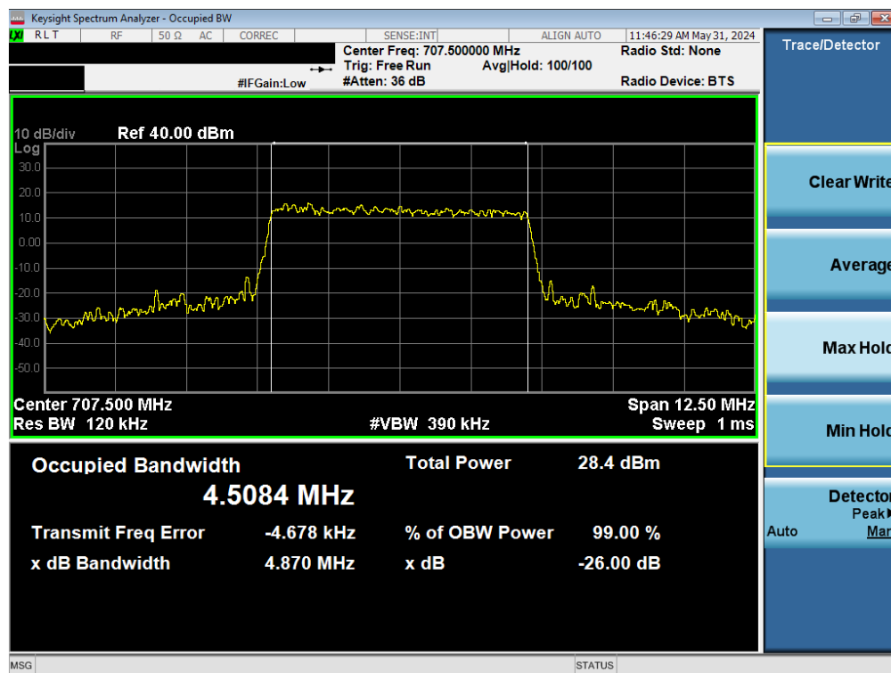
Plot 7-42. Occupied Bandwidth Plot (NR Band n12 - 5MHz CP-OFDM 16-QAM - Full RB – ANT1)
