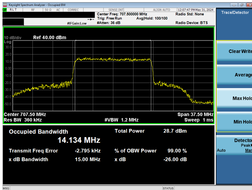
Plot 7-35. Occupied Bandwidth Plot (NR Band n12 - 15MHz QPSK - Full RB – ANT1)
