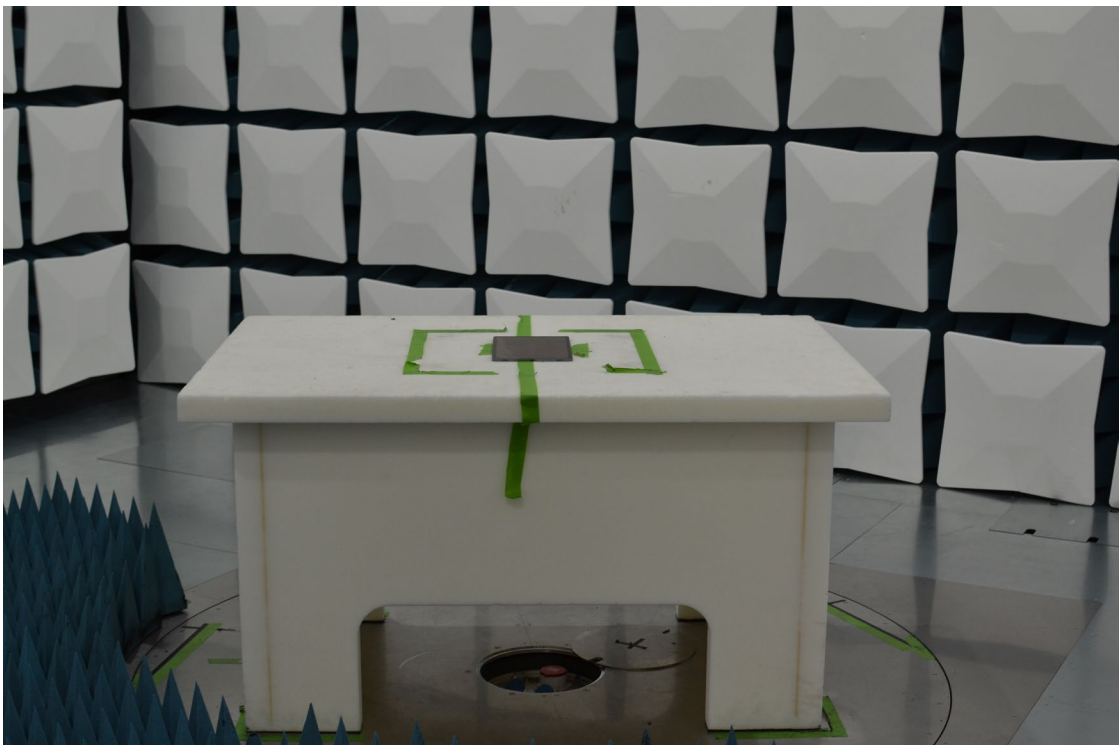
Figure 4. Test Setup – X Position – 30MHz-1GHz
