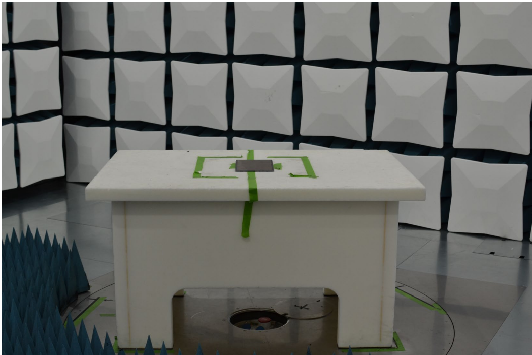
Figure 6. Test Setup – X Position – 30MHz-1GHz
