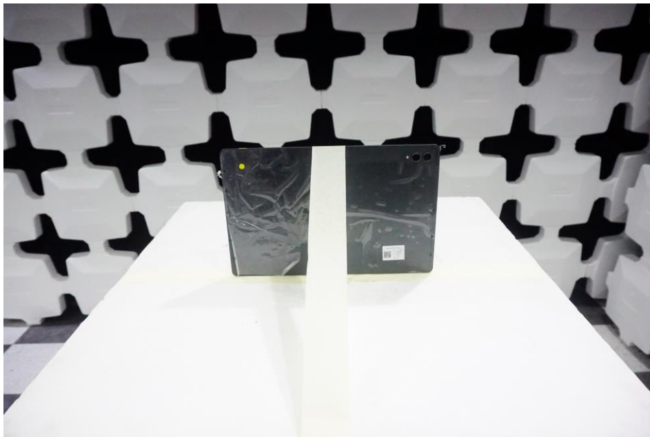
Figure 6. Test Setup – Y Position – 1GHz-18GHz
