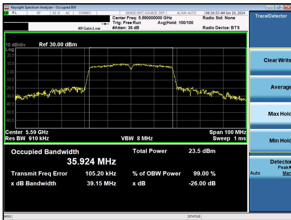
Plot 7-20. 26dB Bandwidth Plot MIMO ANT1 (40MHz BW 802.11n (UNII Band 2C) – Ch. 118)
