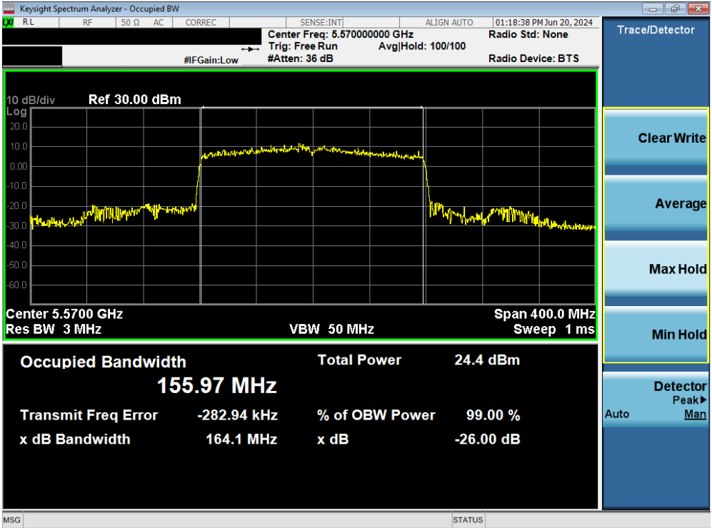
Plot 7-50. 26dB Bandwidth Plot MIMO ANT2 (160MHz BW 802.11be (UNII Band 2C) – Ch. 114)
