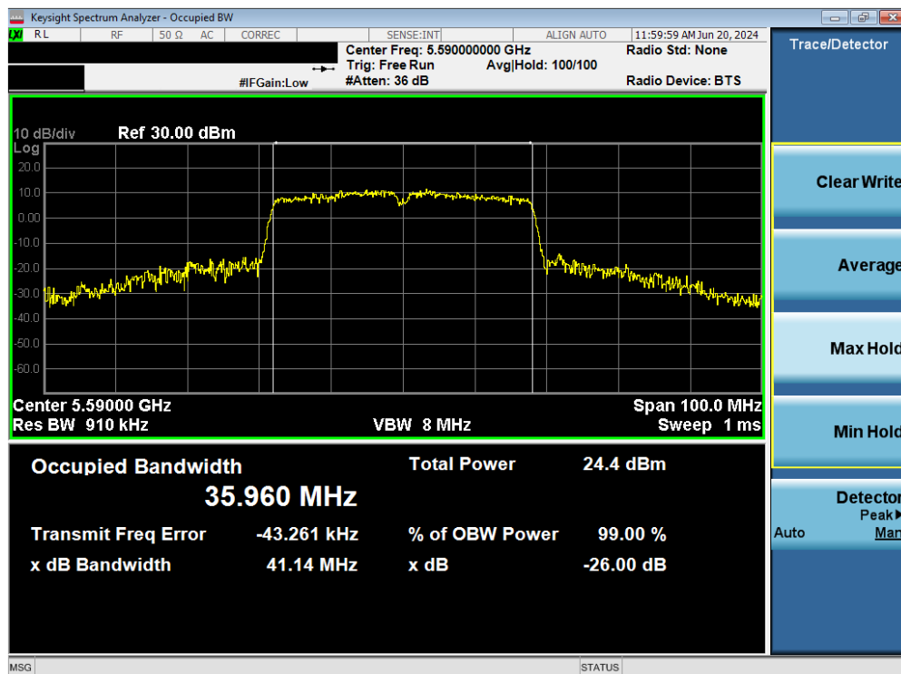
Plot 7-45. 26dB Bandwidth Plot MIMO ANT2 (40MHz BW 802.11n (UNII Band 2C) – Ch. 118)
