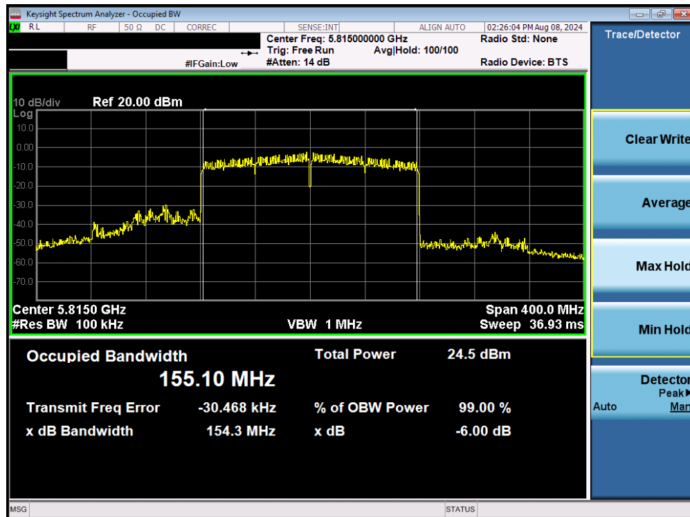
Plot 7-92. 6dB Bandwidth Plot MIMO ANT2 (160MHz BW 802.11be (UNII Band 3/4) – Ch. 163)
