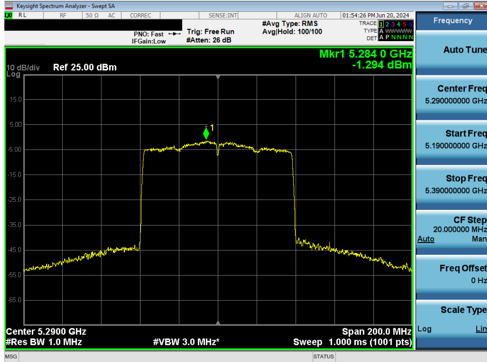
Plot 7-154. Power Spectral Density Plot MIMO ANT2 (80MHz BW 802.11ac (UNII Band 2A) – Ch. 58)
