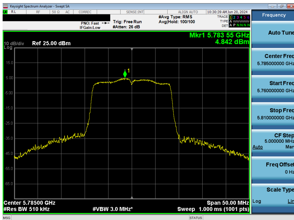
Plot 7-165. Power Spectral Density Plot MIMO ANT2 (802.11a (UNII Band 3) – Ch. 157)
