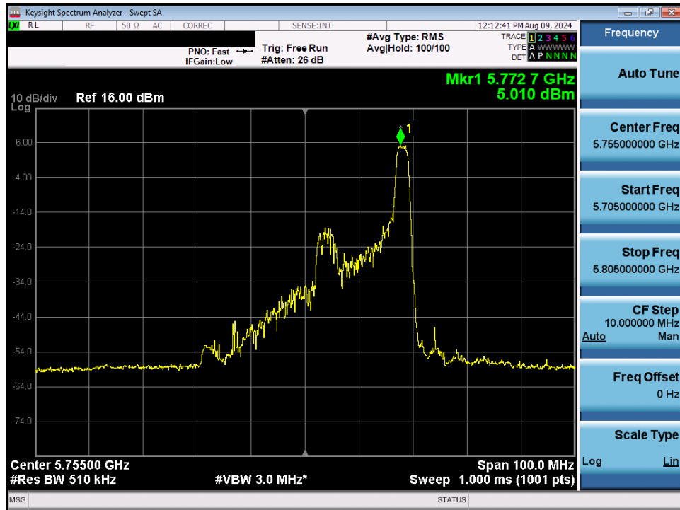
Plot 7-121. Power Spectral Density Plot MIMO ANT1 (40MHz BW 802.11be – 26 Tones (UNII Band 3) – Ch. 151)
