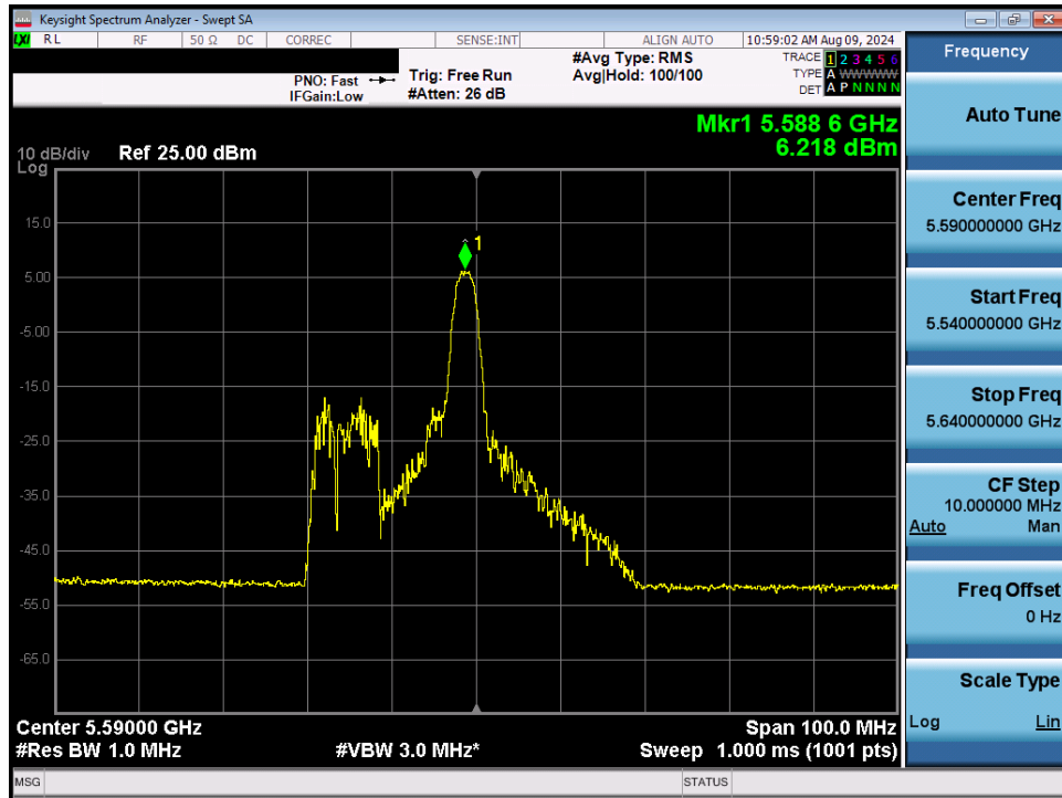
Plot 7-171. Power Spectral Density Plot MIMO ANT2 (40MHz BW 802.11be – 26 Tones (UNII Band 2C) – Ch. 118)
