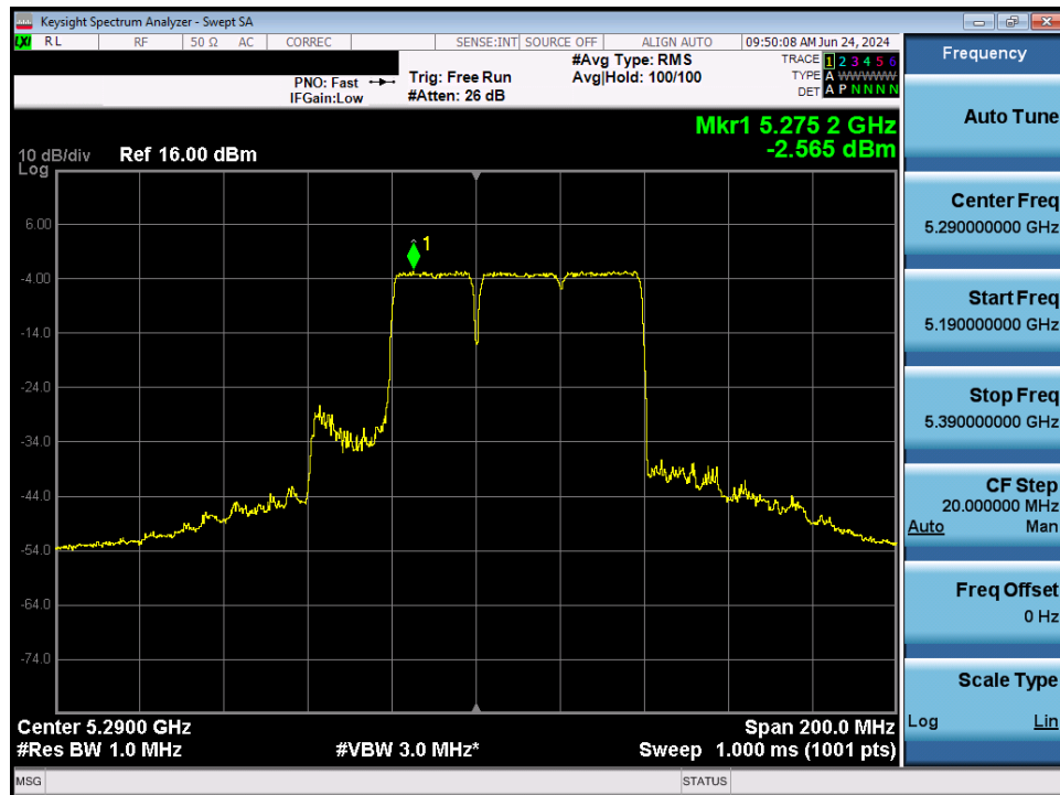
Plot 7-151. Power Spectral Density Plot MIMO ANT1 (80MHz BW 802.11be – 484+242Tones (UNII Band 2A) – Ch. 58)
