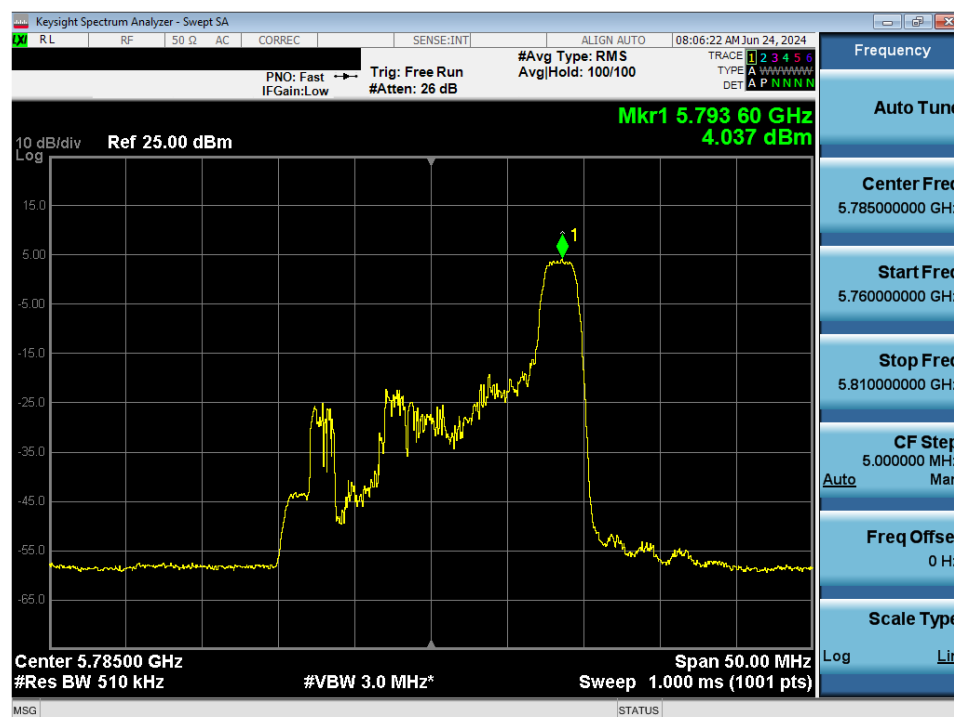
Plot 7-174. Power Spectral Density Plot MIMO ANT2 (20MHz BW 802.11be – 26 Tones (UNII Band 3) – Ch. 157)
