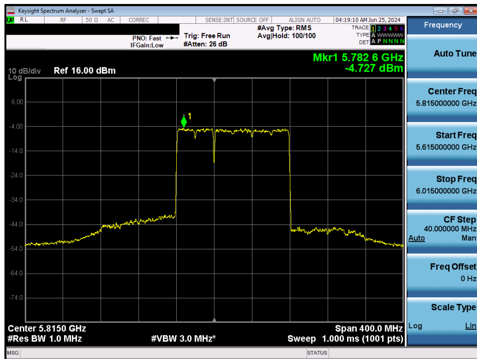
Plot 7-162. Power Spectral Density Plot MIMO ANT1 (160MHz BW 802.11be – 996+484 Tones (UNII Band 3/4) – Ch. 163)
