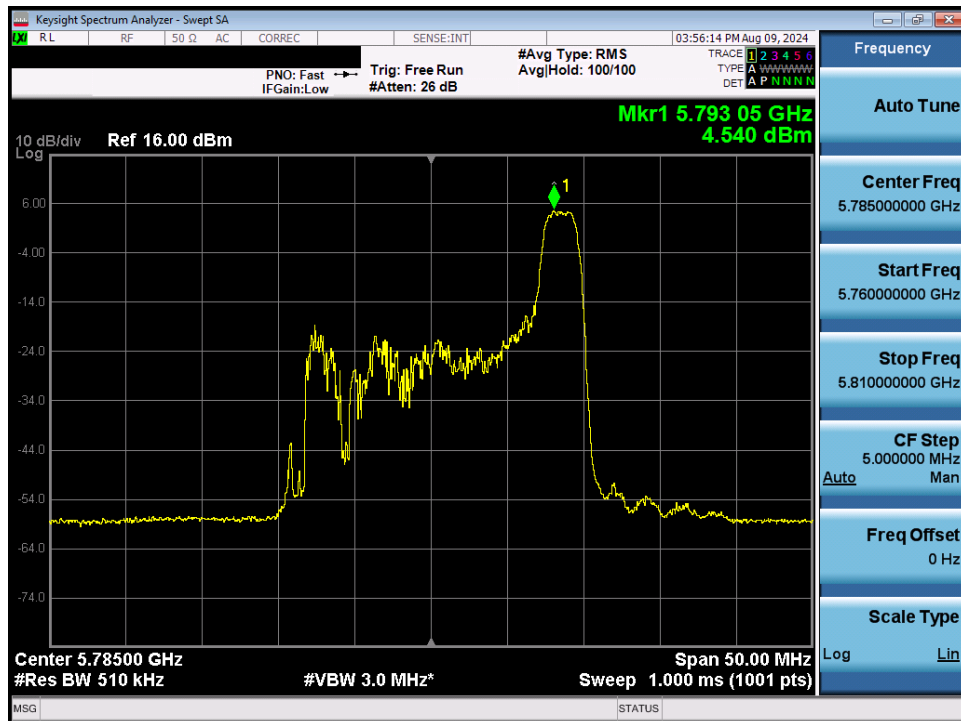
Plot 7-120. Power Spectral Density Plot MIMO ANT1 (20MHz BW 802.11be – 26 Tones (UNII Band 3) – Ch. 157)
