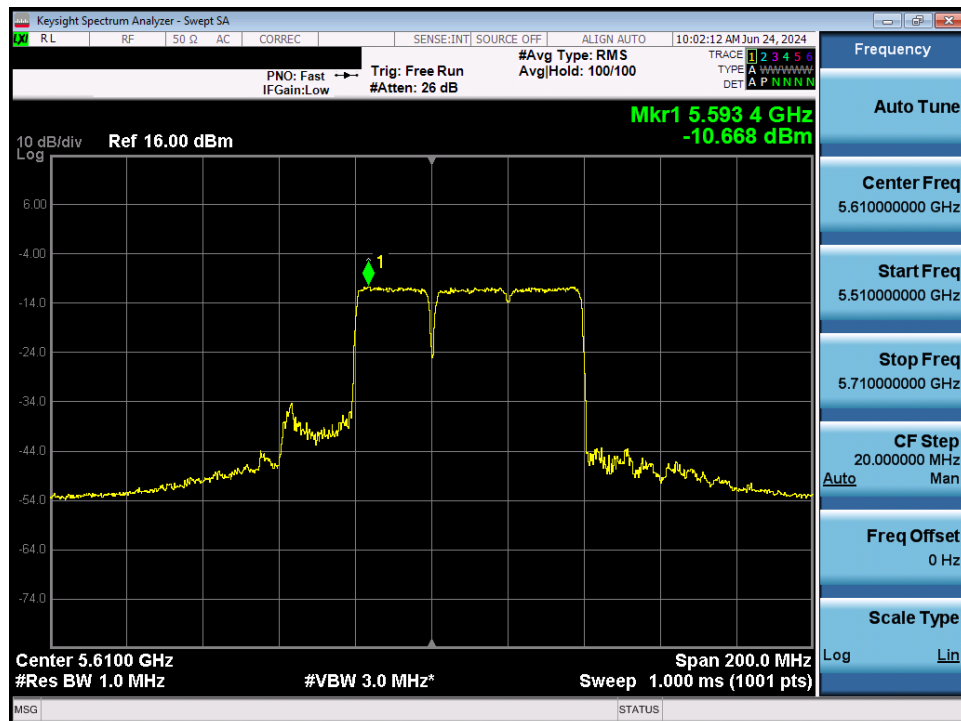
Plot 7-154. Power Spectral Density Plot MIMO ANT1 (80MHz BW 802.11be – 484+242Tones (UNII Band 2C) – Ch. 122)
