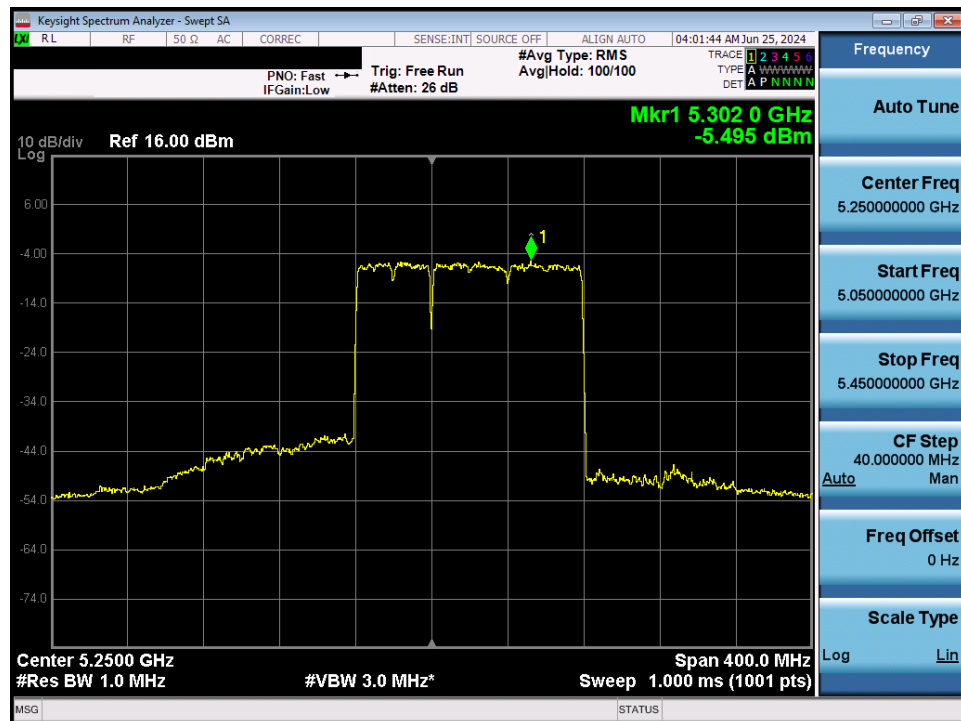
Plot 7-148. Power Spectral Density Plot MIMO ANT1(160MHz BW 802.11be – 996+484 Tones (UNII Band 1/2A) – Ch. 50)
