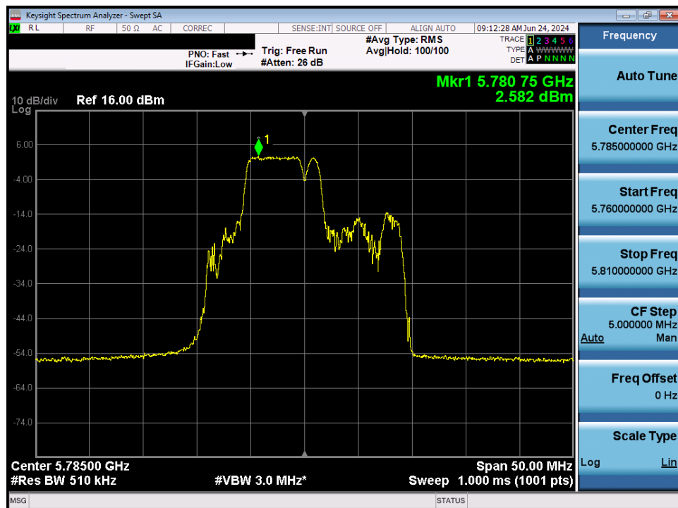
Plot 7-156. Power Spectral Density Plot MIMO ANT1 (20MHz BW 802.11be – 52+26 Tones (UNII Band 3) – Ch. 157)
