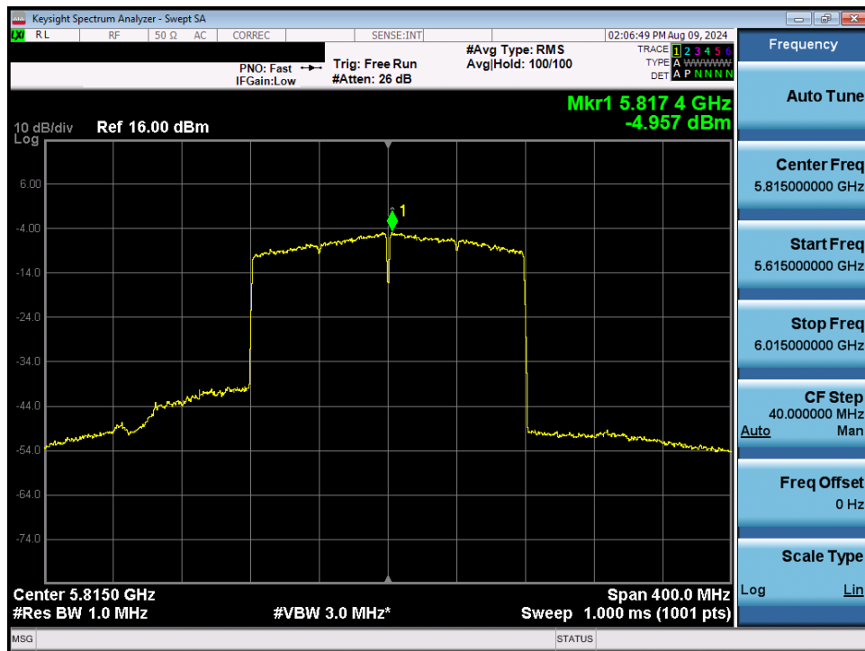
Plot 7-144. Power Spectral Density Plot MIMO ANT1 (160MHz BW 802.11be – 996*2 Tones (UNII Band 3/4) – Ch. 163)
