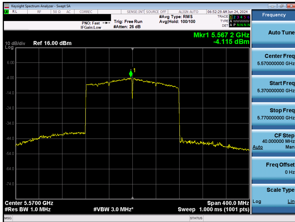
Plot 7-137. Power Spectral Density Plot MIMO ANT1 (160MHz BW 802.11be – 2x996 Tones (UNII Band 2C) – Ch. 114)
