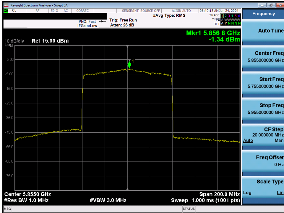
Plot 7-143. Power Spectral Density Plot MIMO ANT1 (80MHz BW 802.11be – 996 Tones (UNII Band 3/4) – Ch. 171)
