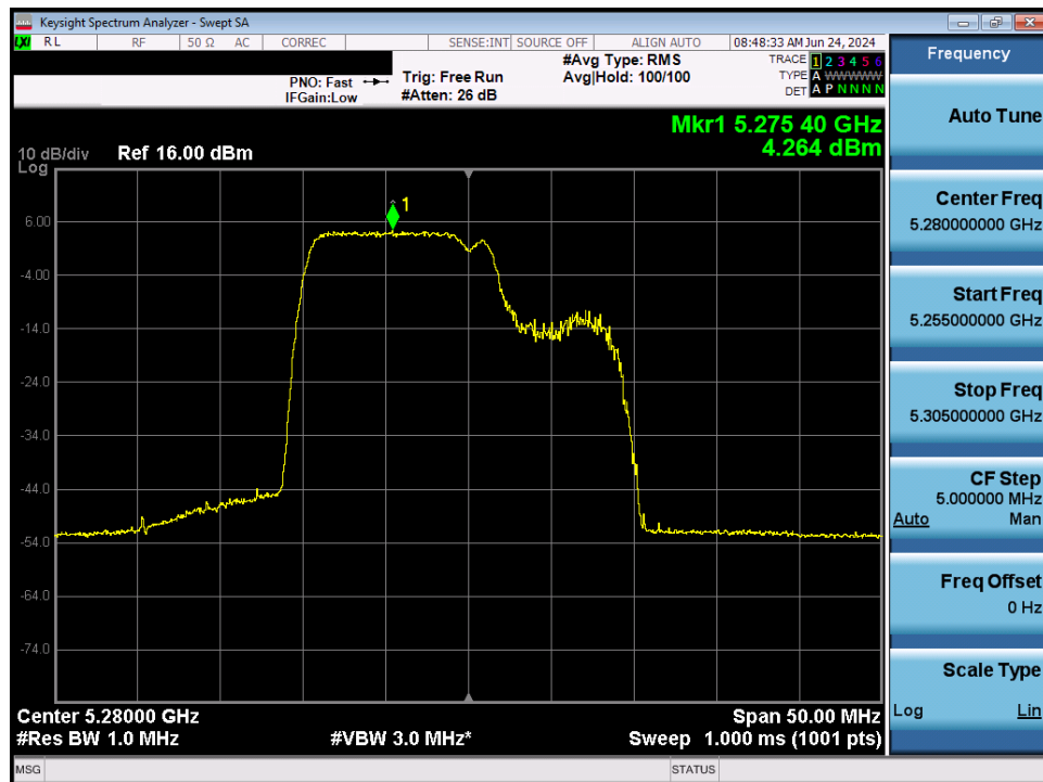
Plot 7-150. Power Spectral Density Plot MIMO ANT1 (20MHz BW 802.11be – 106+26 Tones (UNII Band 2A) – Ch. 56)
