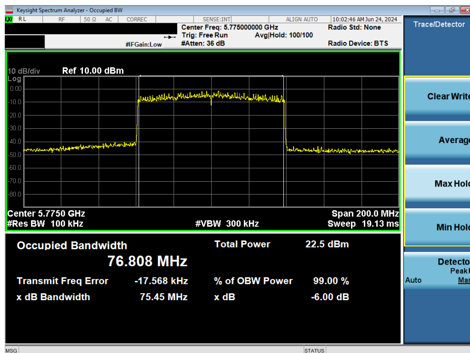
Plot 7-97. 6dB Bandwidth Plot MIMO ANT2 (80MHz BW 802.11be – 996 Tones (UNII Band 3) – Ch. 155)
