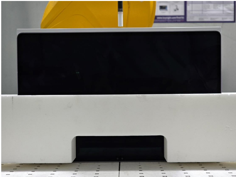
SAR Test Setup Photo 22 – Tablet with Keyboard Variant 1, Left Edge at 2 mm
