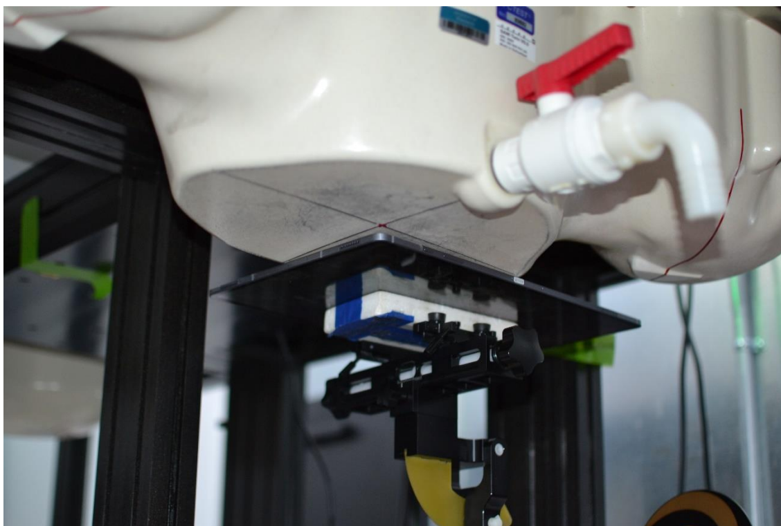
SAR Test Setup Photo 6 – Tablet, Back Side at 0 mm – Antenna WIFI 2
