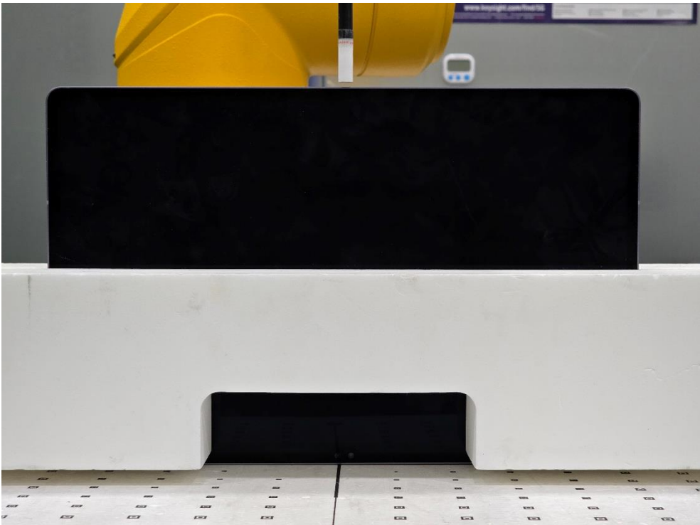
SAR Test Setup Photo 28 – Tablet, Left Edge at 2 mm
