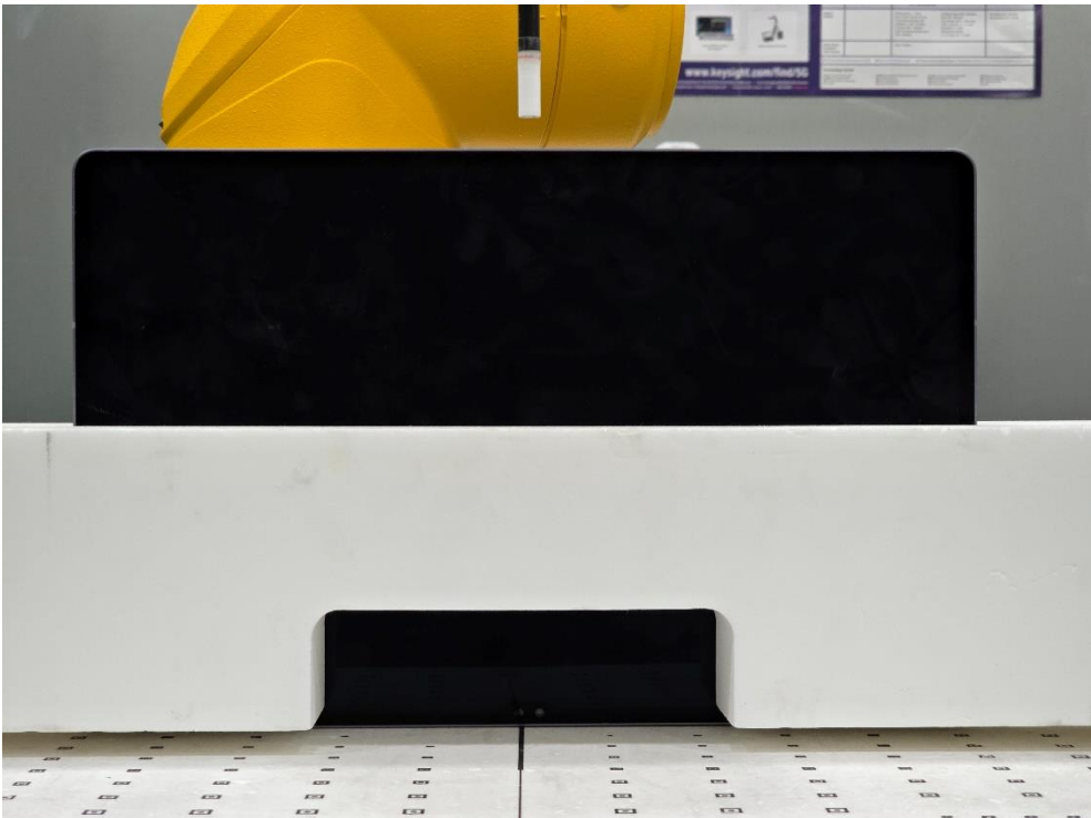
SAR Test Setup Photo 29 – Tablet, Left Edge at 8.46 mm
