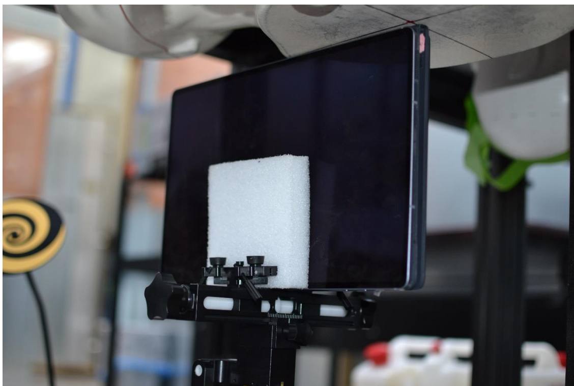
SAR Test Setup Photo 12 – Tablet with Keyboard Variant 1, Left Edge at 0 mm – Antenna WIFI 1, 2
