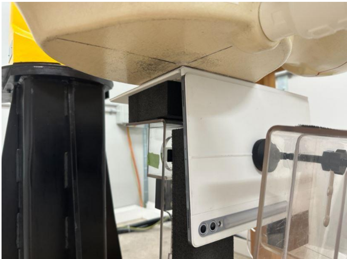
SAR Test Setup Photo 20 – Laptop with Keyboard Variant 1, Bottom Edge at 0 mm Antenna WIFI 1, 2
