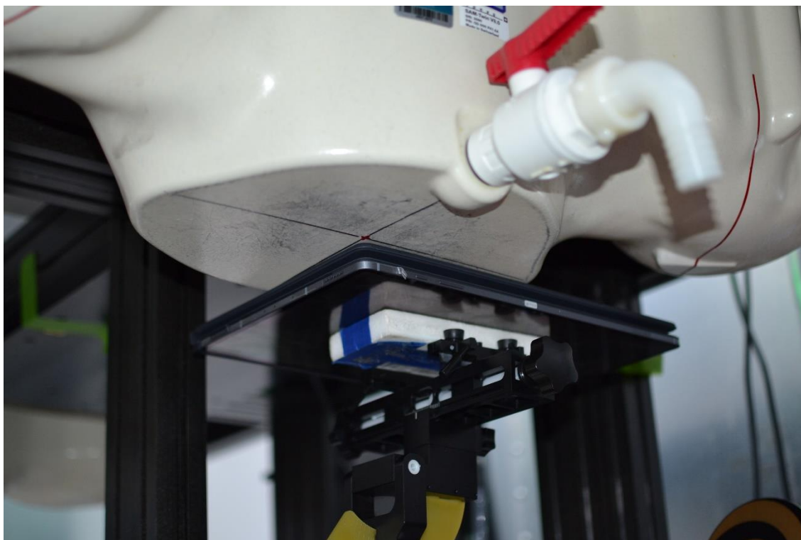
SAR Test Setup Photo 7 – Tablet with Keyboard Variant 1, Back Side at 0 mm – Antenna WIFI 2
