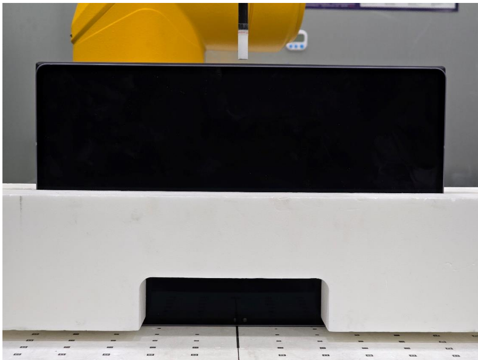
SAR Test Setup Photo 23 – Tablet with Keyboard Variant 2, Left Edge at 2 mm
