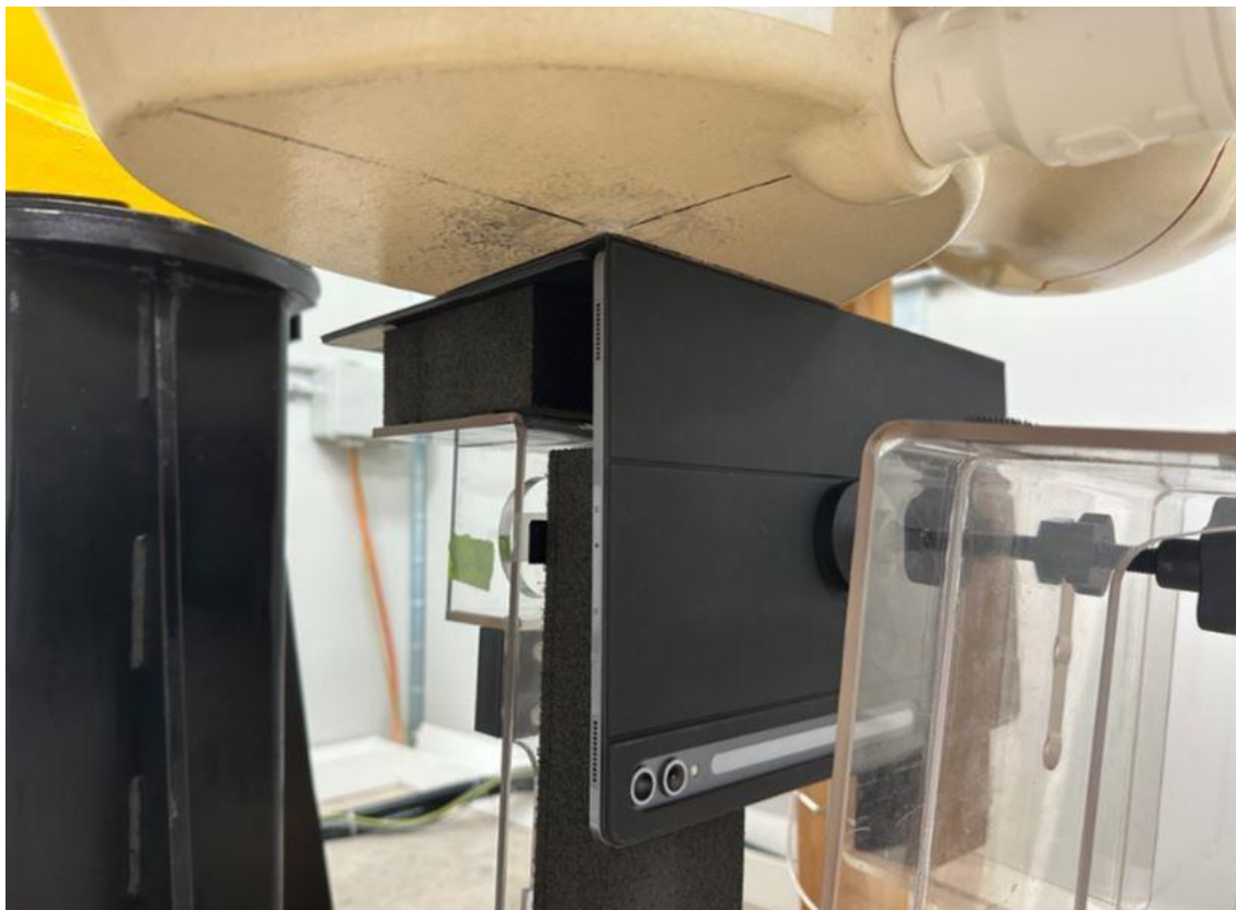
SAR Test Setup Photo 21 – Laptop with Keyboard Variant 2, Bottom Edge at 0 mm Antenna WIFI 1, 2
