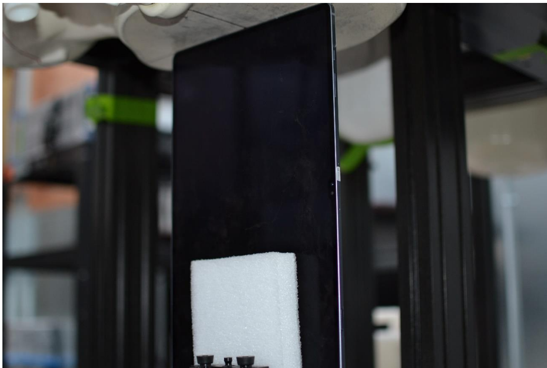
SAR Test Setup Photo 19 – Tablet, Top Edge at 20 mm – Antenna WIFI 1, 2
