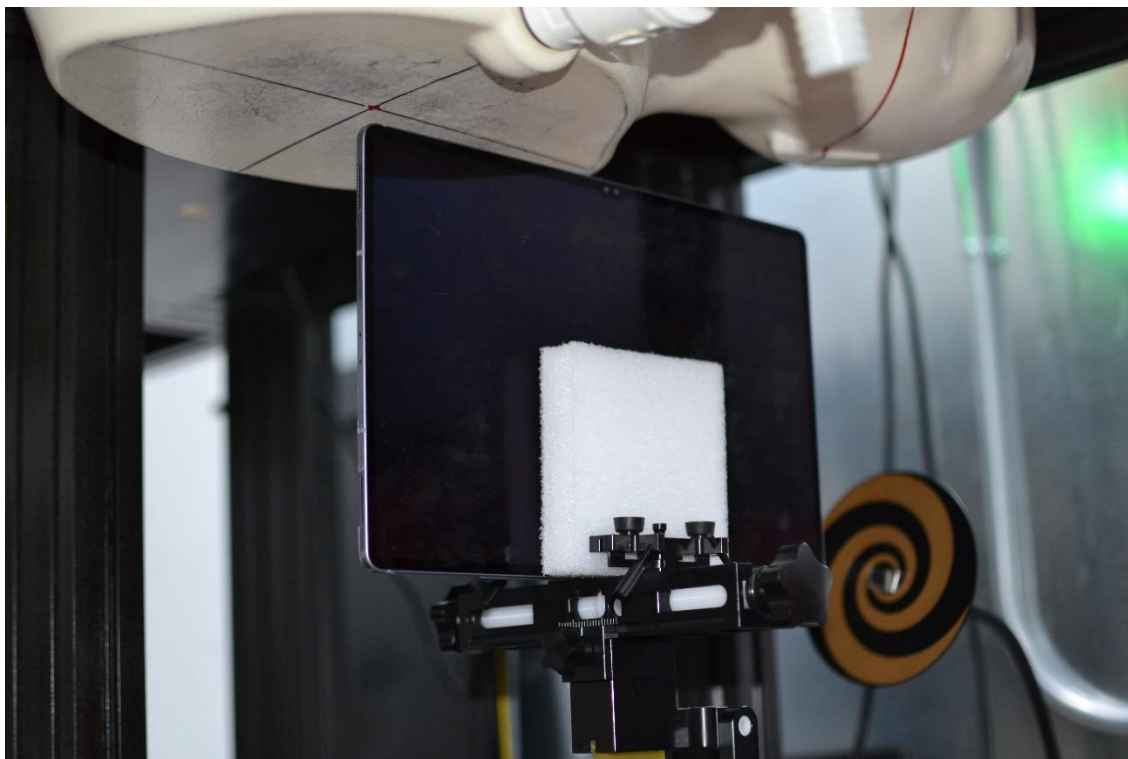
SAR Test Setup Photo 13 – Tablet, Right Edge at 7 mm – Antenna WIFI 1, 2
