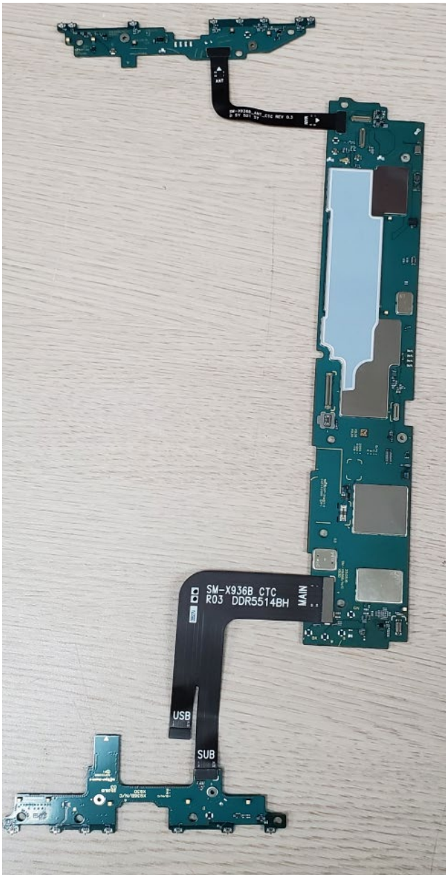
Main and Sub PBAs front
