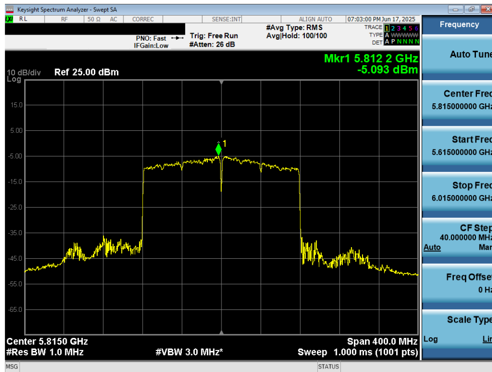
Plot 7-113. Power Spectral Density Plot MIMO ANT2 (160MHz BW 802.11be – 996*2 Tones (UNII Band 3/4) – Ch. 163)
