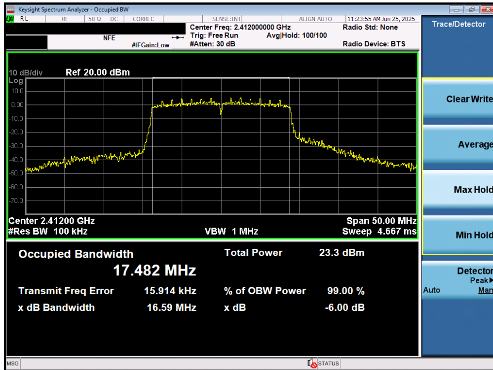
Plot 7-7. 6dB Bandwidth Plot MIMO ANT1 (802.11n/ac (2.4GHz) – Ch. 1)
