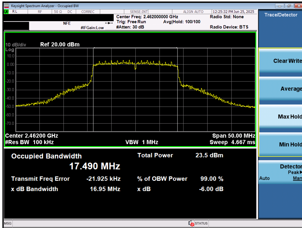
Plot 7-21. 6dB Bandwidth Plot MIMO ANT2 (802.11n/ac (2.4GHz) – Ch. 11)
