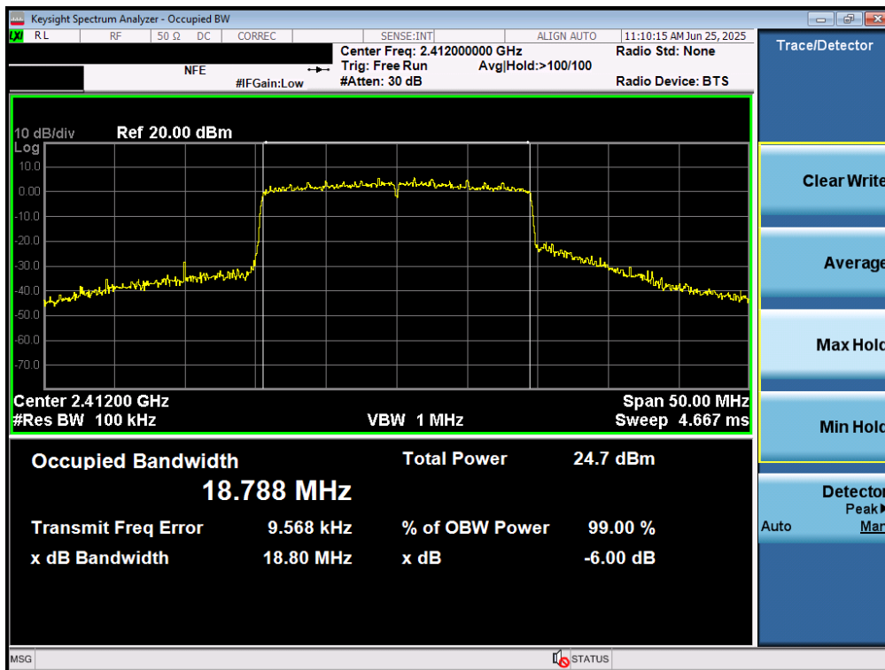
Plot 7-10. 6dB Bandwidth Plot MIMO ANT1 (802.11ax/be (2.4GHz) – Ch. 1)
