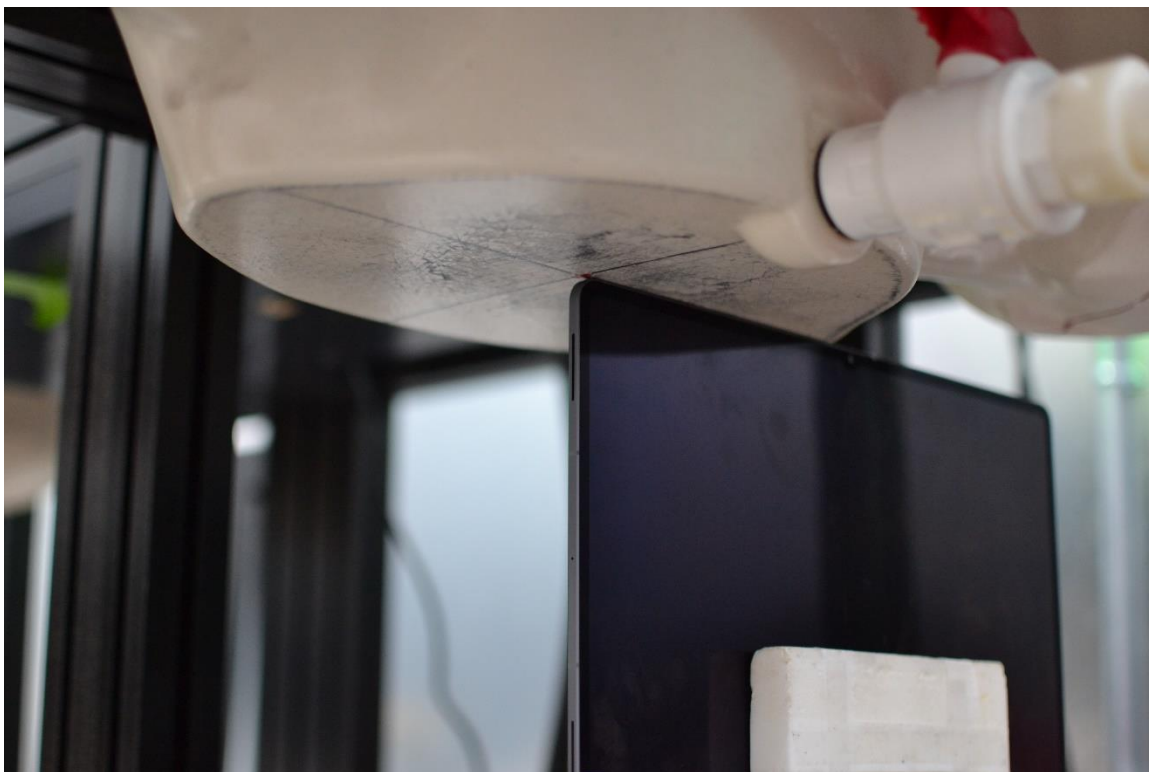
SAR Test Setup Photo 11 – Tablet, Right Edge at 0 mm
