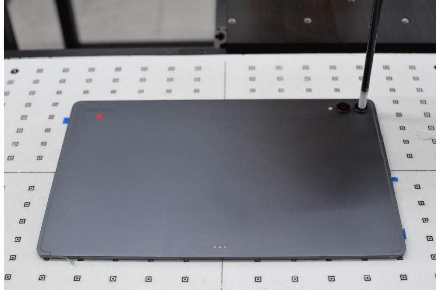
SAR Test Setup Photo 20 – Tablet, Back Side at 2 mm – Antenna WIFI 1
