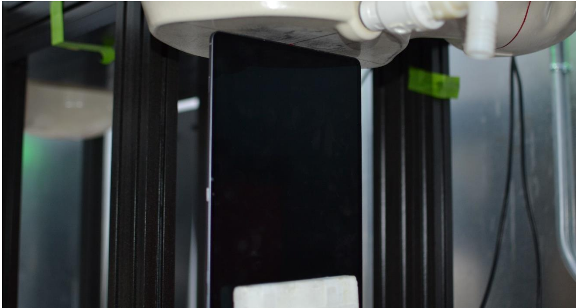
SAR Test Setup Photo 9 – Tablet, Bottom Edge at 0 mm
