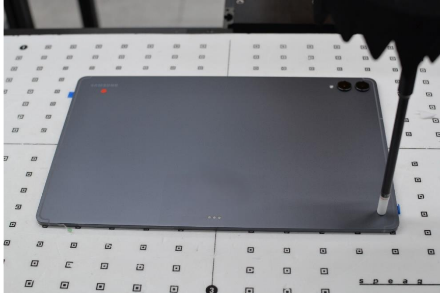
SAR Test Setup Photo 18 – Tablet, Back Side at 2 mm – Antenna WIFI 0
