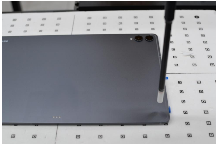
SAR Test Setup Photo 19 – Tablet, Back Side at 9.95 mm– Antenna WIFI 0
