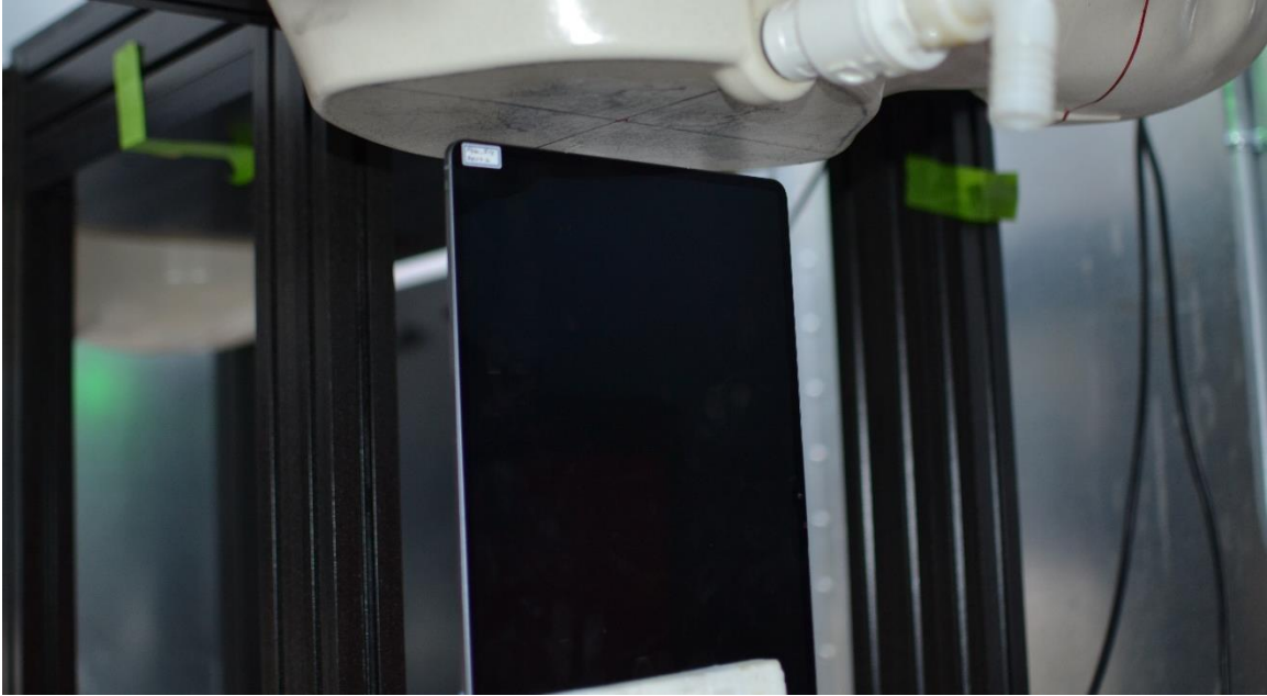
SAR Test Setup Photo 7 – Tablet, Top Edge at 19 mm
