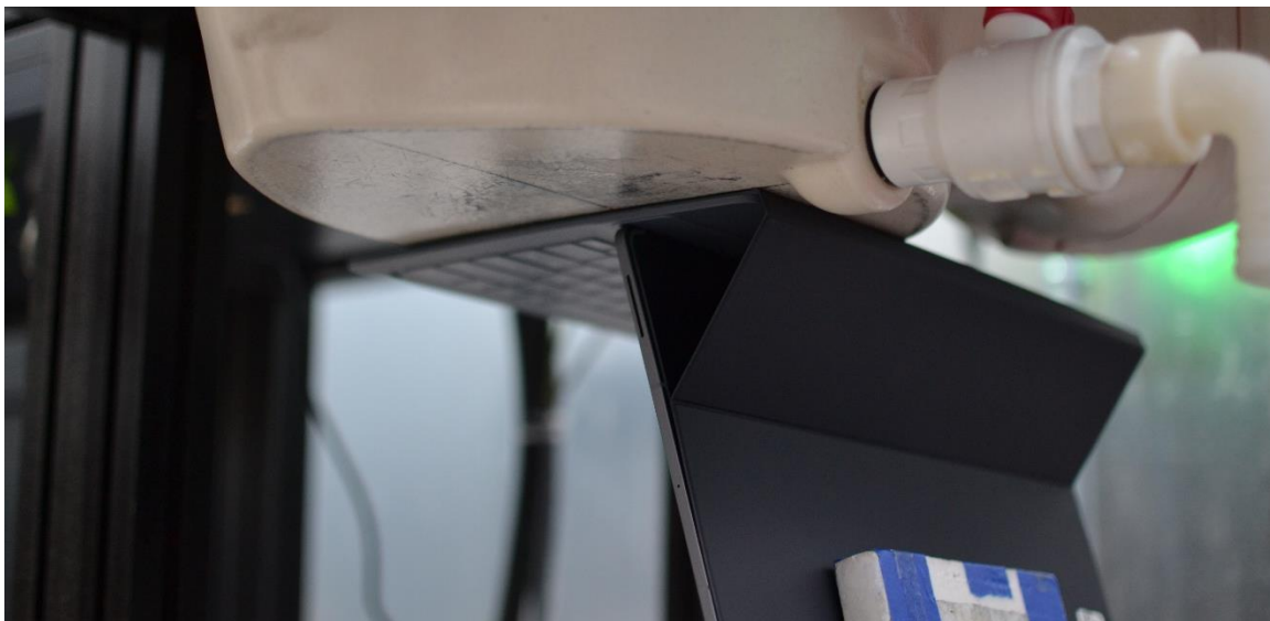
SAR Test Setup Photo 16 – Laptop with Keyboard, Bottom Edge at 0 mm
