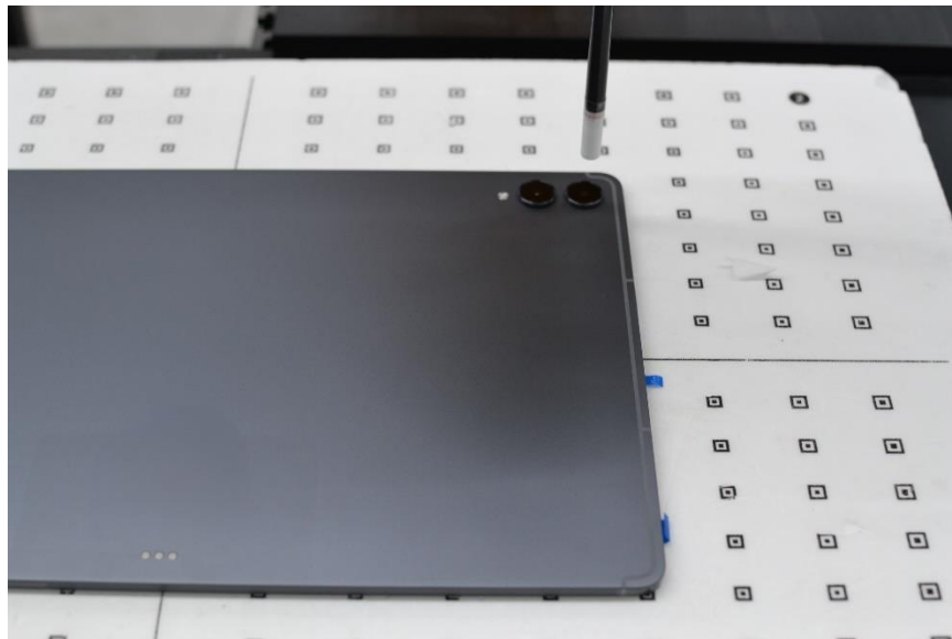
SAR Test Setup Photo 21 – Tablet, Back Side at 9.95 mm– Antenna WIFI 1
