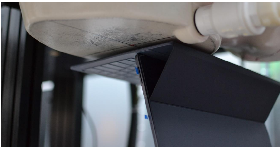
SAR Test Setup Photo 17 – Laptop with Keyboard, Bottom Edge at 9 mm
