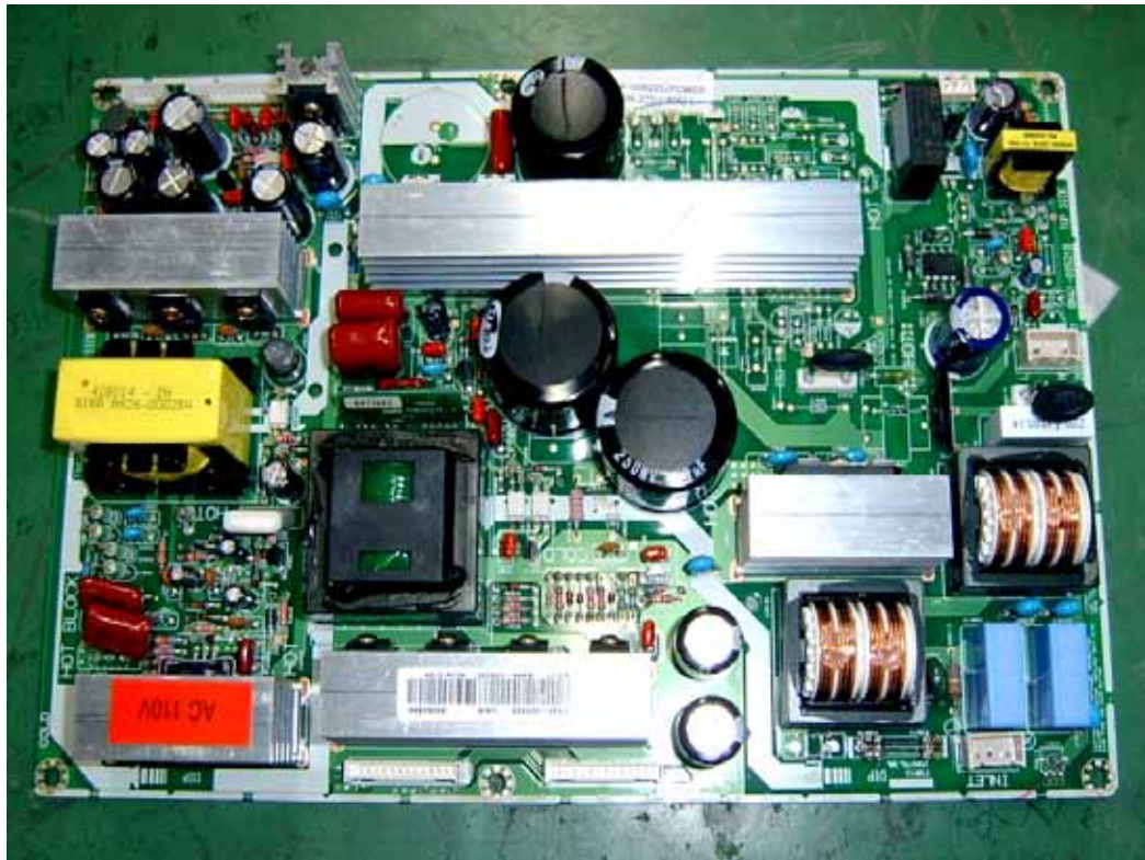
SMPS board top view
