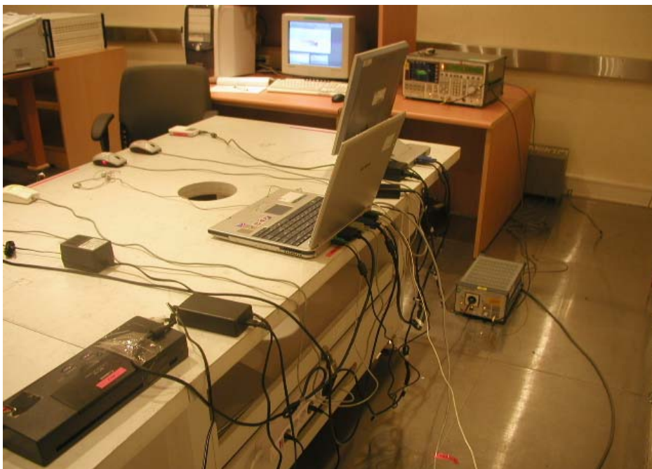
Pic. 2 Conducted Emission (Rear)
