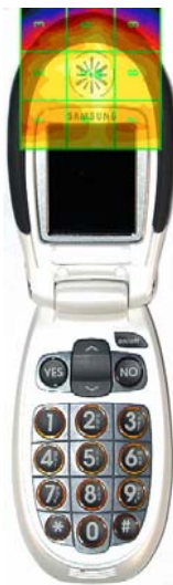
Figure 27 Sample E-field Scan Overlay
