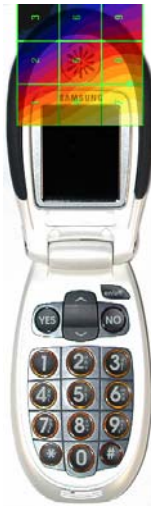
Figure 28 Sample H-field Scan Overlay
