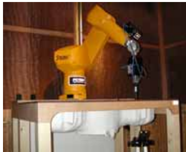
Figure 3-2 DASY4 SAR Measurement System
