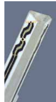
Figure 4-2 Probe Thick Film Technique
