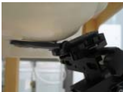
Figure 8.2 Right Head SAR Test Setup
