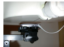
Figure 14.14 Body SAR Test Setup -- w/o Holster --
