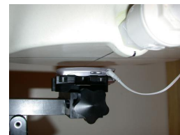
Figure 14.15 Body SAR Test Setup -- w/o Belt-clip --
