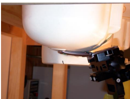
Figure 14.1 Right Head SAR Test Setup -- Cheek / Touch Position --
