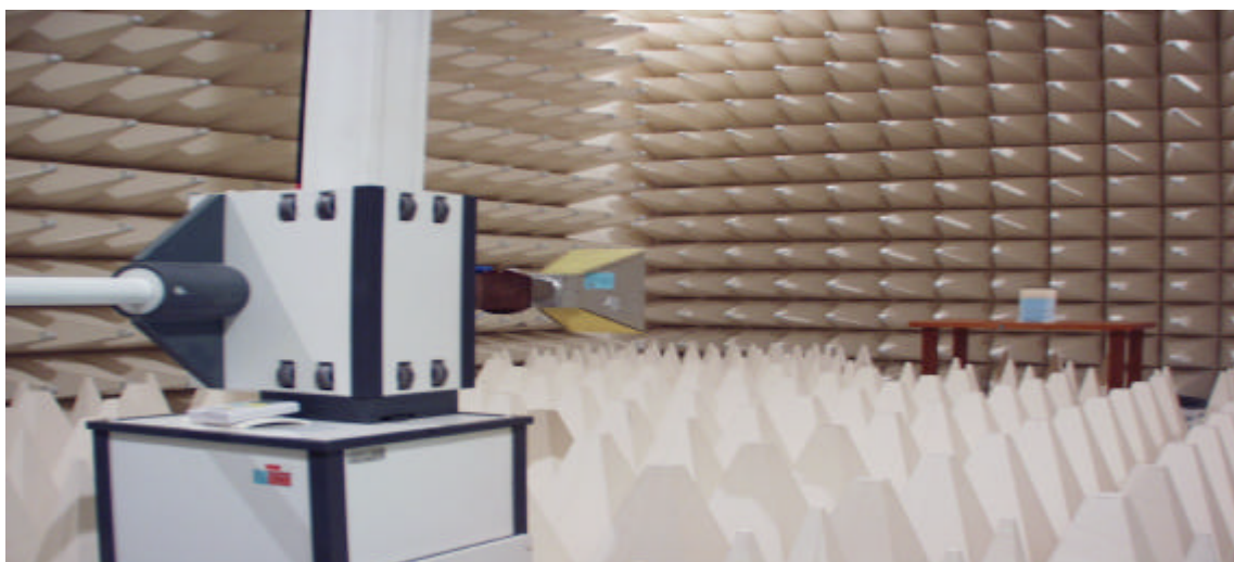
Figure2. Photograph of 3m Fully Anechoic Chamber
